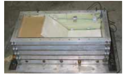
2c. Clay liner placed
