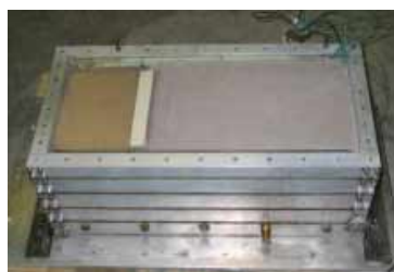
2d. Accelerometers placed on clay liner
