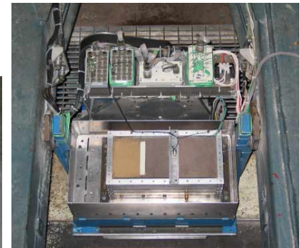
2f. Model loaded in centrifuge
