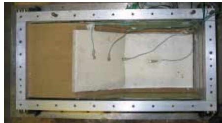
2d. Accelerometers placed on clay liner
