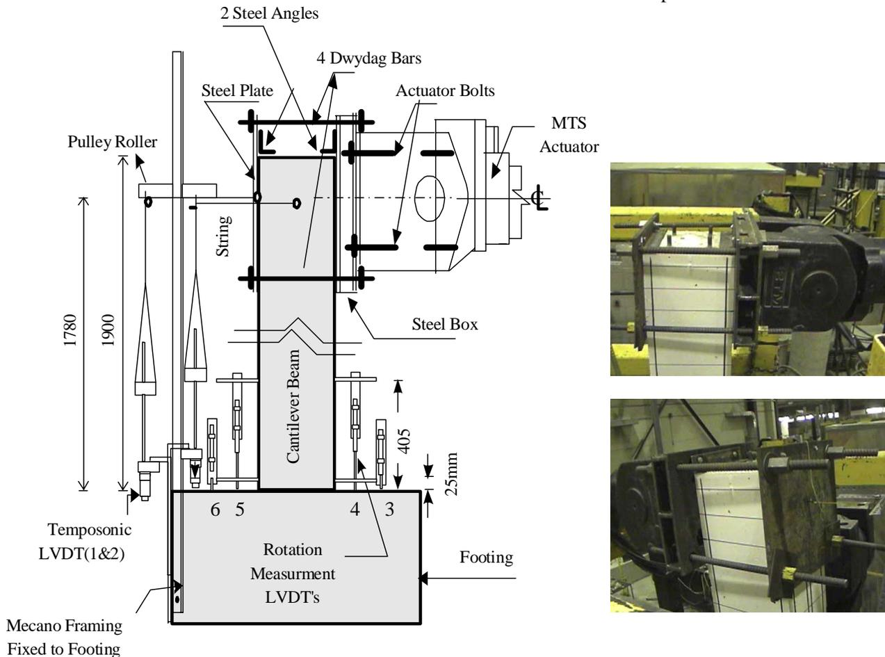
**Figure 7 Application of lateral load on beams and typical instrumentation**
