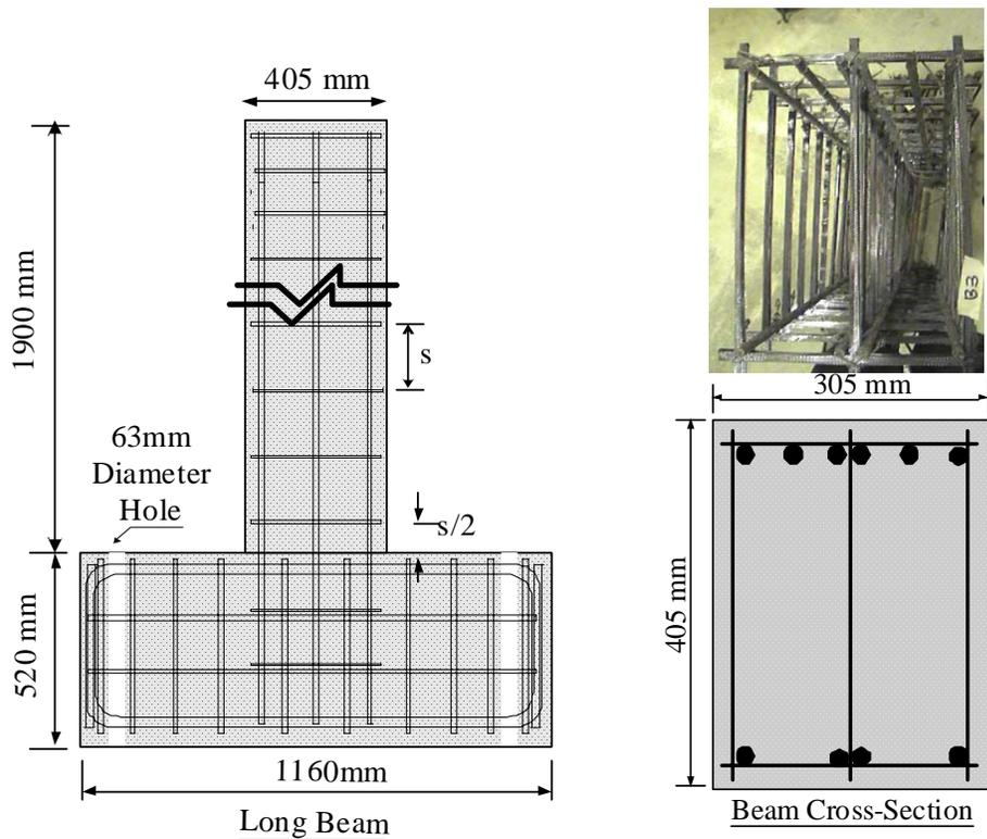
**Figure 2 Details of beam specimens**
