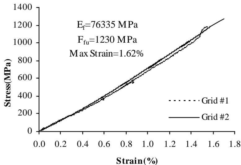
**Figure 4 Stress-strain relationships for NEFMAC grids**
