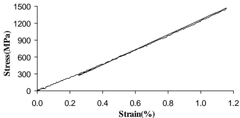
**Figure 3 Stress-strain relationship of Pultral FRP bars**
