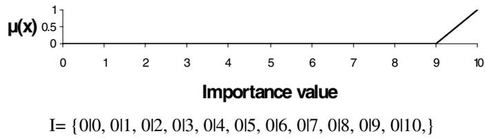
**Figure 4.** Function of weight of  $K_1$  (year of project and construction of the bridge).
