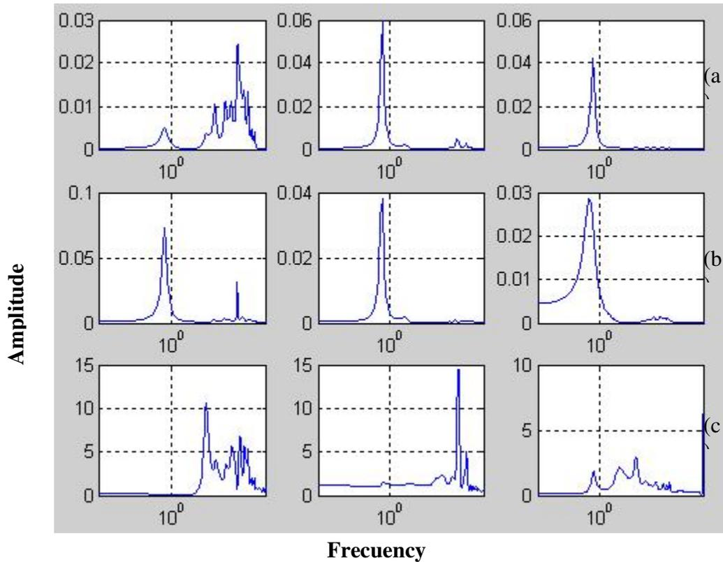
**Figure 7.** Fourier spectra (a) bridge, (b) free field and (c) transference function. The first column show longitudinal component, the second one the vertical and the third one is the transversal component.
