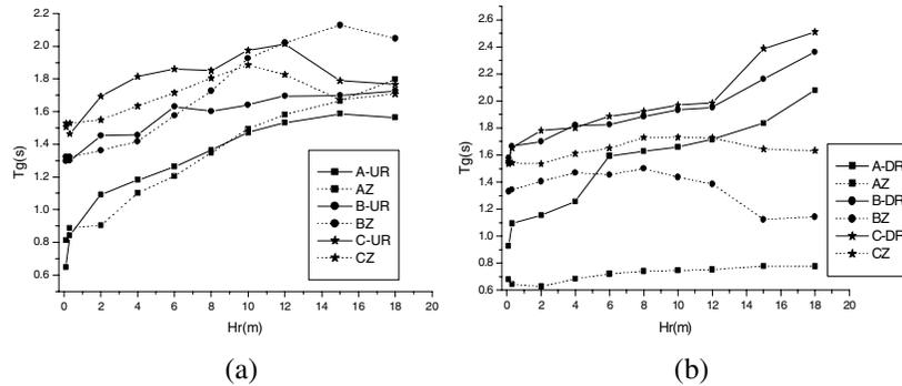
**Figure 7 Comparison between profiles with soft interlayer at the top and bottom and normal profiles**
