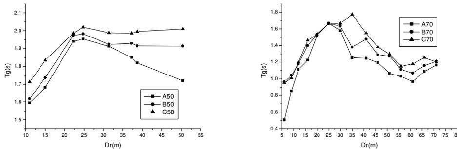
**Figure 6** the effects of imbedded depths of soft interlayer on  $T_g$  s
