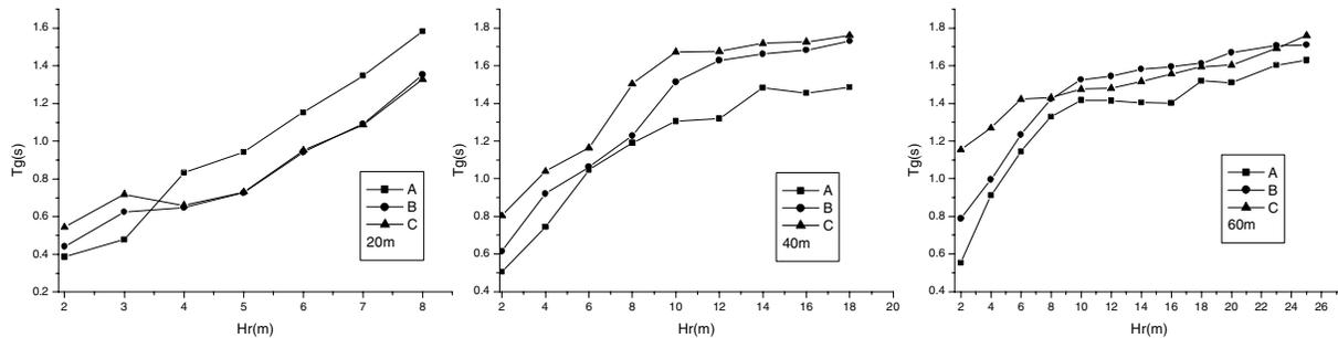
**Figure 4** the effects of thicknesses of soft surface layer on  $T_g$  s
