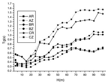
**Figure 3 the effects of soft surface layer on  $T_g$  s under different H**
