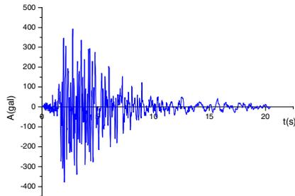
Figure 1 acceleration input ground motion(C time history)
