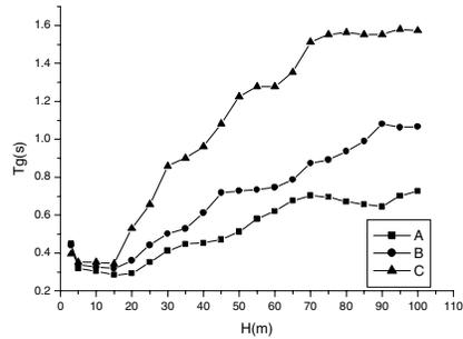
**Figure 2 the effects of overlying layer's thicknesses on  $T_g$  s**
