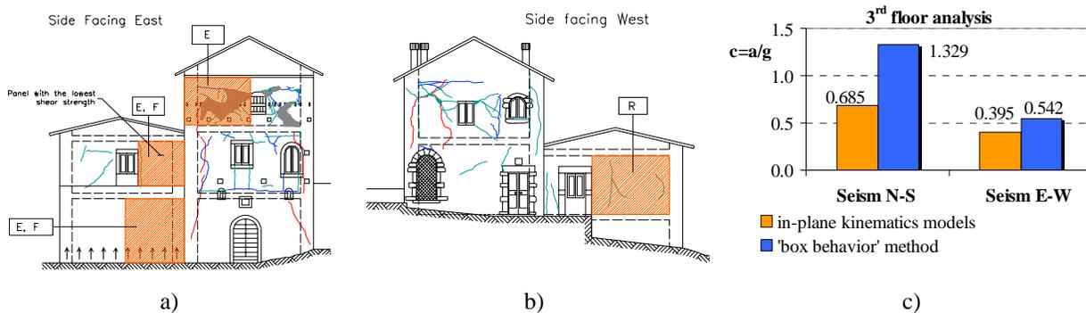
Figure 11: Results of method adopting the “box behavior” of the structure: (a) the most damaged panels (East side) are given as simply reaching the elastic (E) or first crack limit (F), whereas the panel led to rupture (R) belong to a very low damaged wall (b); comparison between the two methods (c).
