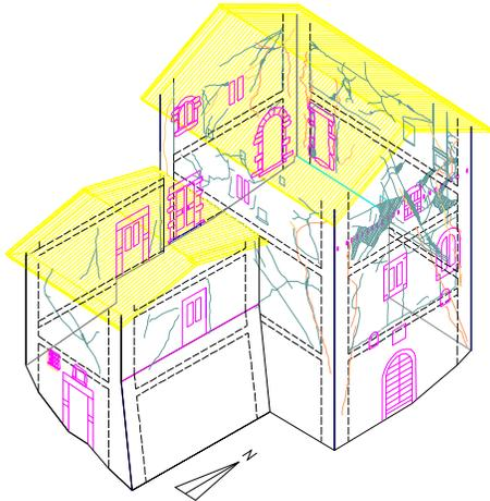
Figure 8: View of the building with survey of the crack pattern: the most damaged portions are the Eastern wall and the Nord-Eastern corner (overturning effects).
