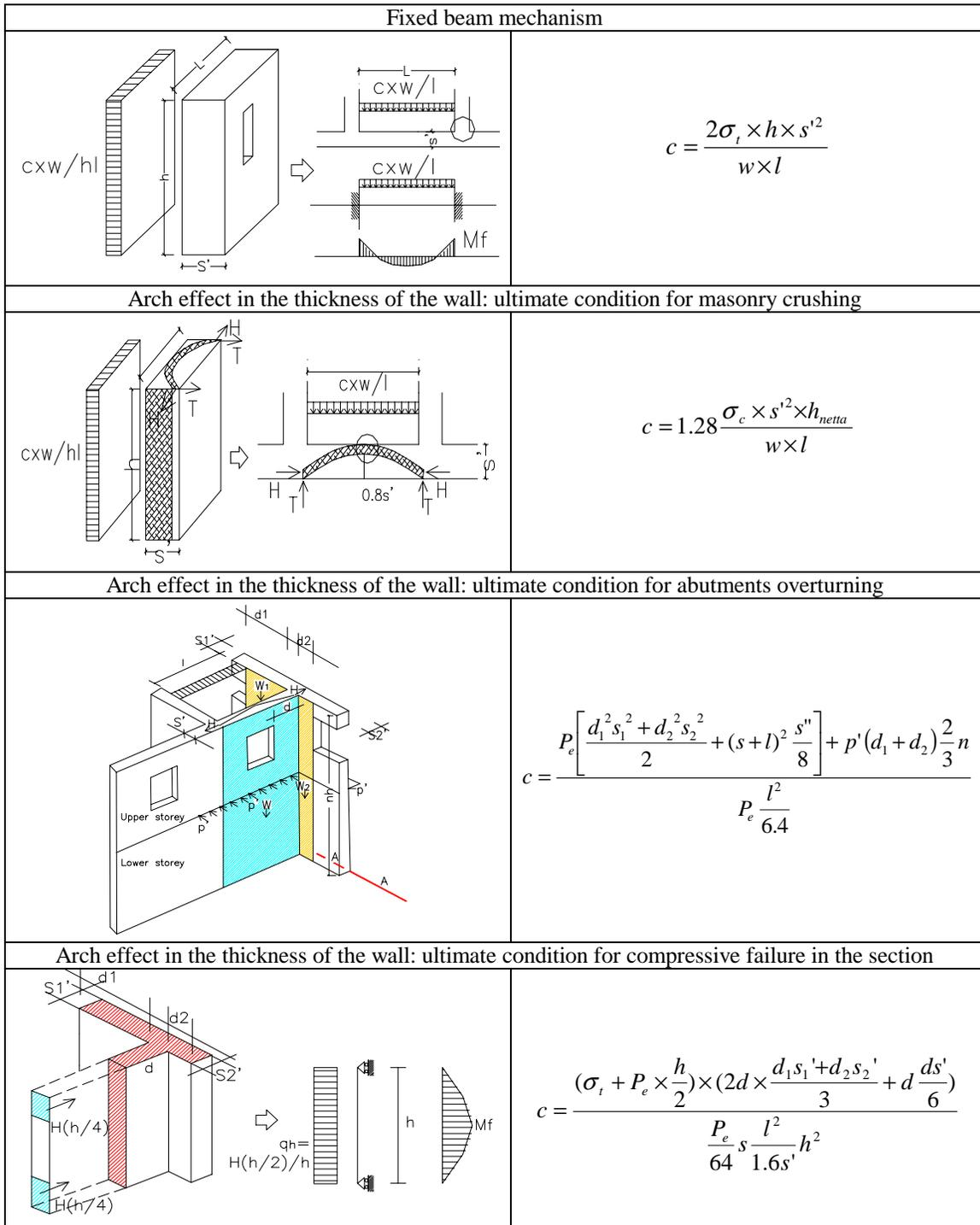
Figure 7: Kinematics models for out-of-plane mechanisms: horizontal strips (Bernardini et al. [8]).
