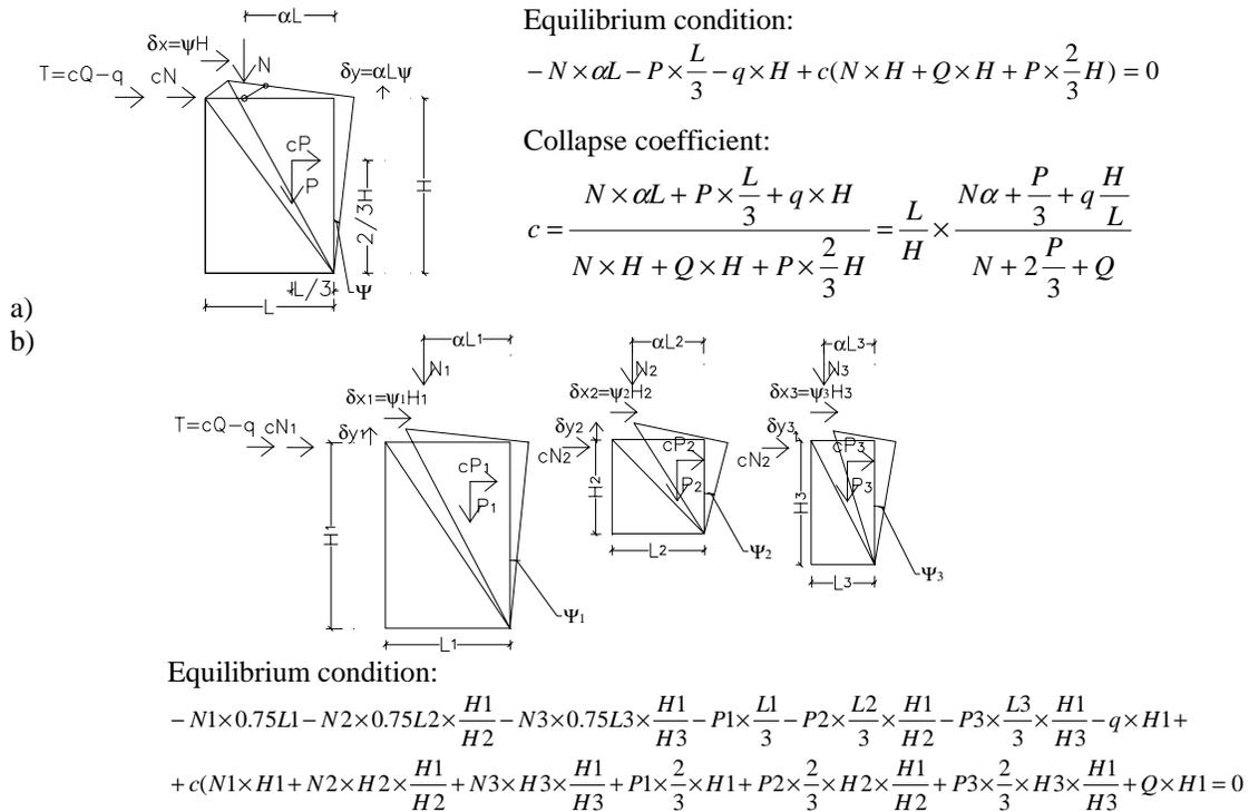
Figure 5: Scheme of the in-plane kinematics model for a wall under in-plane actions: a) single wall, b) multiple-wall system (Giuffrè [5]).
