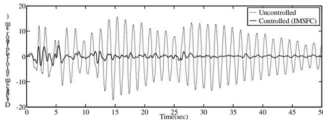
**Figure 8. Controlled and uncontrolled displacement responses of the top floor (El Centro case)**
