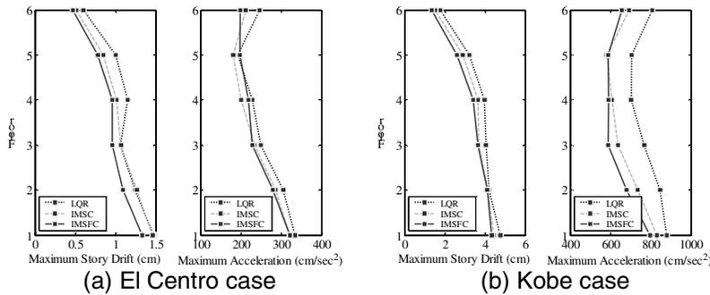
**Figure 9. Maximum story drift and maximum acceleration response**
