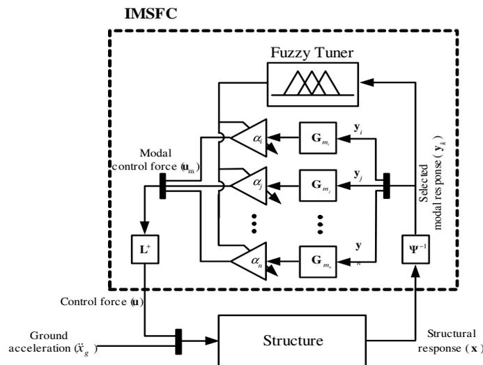
Figure 4. Schematic block diagram of IMSFC
