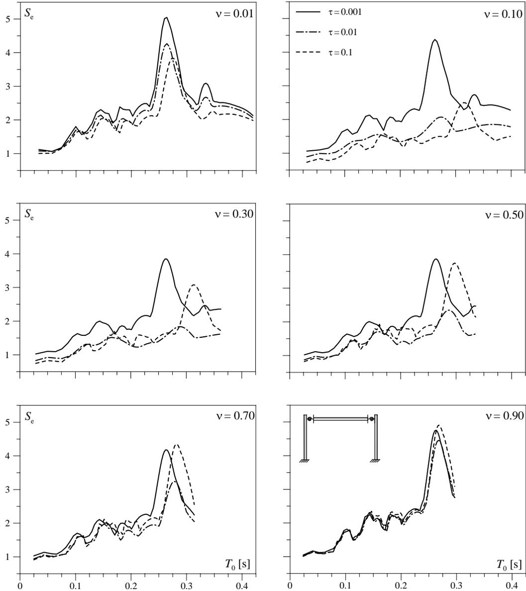
**Fig. 11 – Response spectra of a SDOF frame with viscoelastic joints for the 1976 Friuli earthquake**
