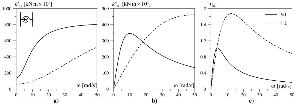
Fig. 5 – Storage modulus (a), loss modulus (b), and loss factor (c) of the viscoelastic hinges
