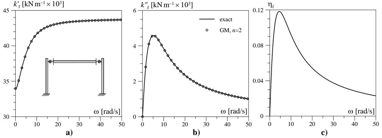
**Fig. 8 – Storage modulus (a), loss modulus (b), and loss factor (c) of the portal frame with viscoelastic joints**
