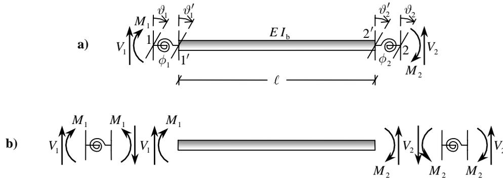
Fig. 2 – Elastic beam with viscoelastic hinges: a) global scheme; b) disassembled components
