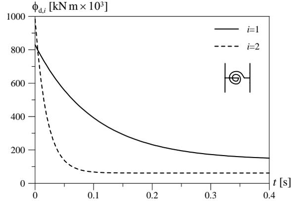
Fig. 4 – Relaxation functions of the viscoelastic hinges at the beam ends
