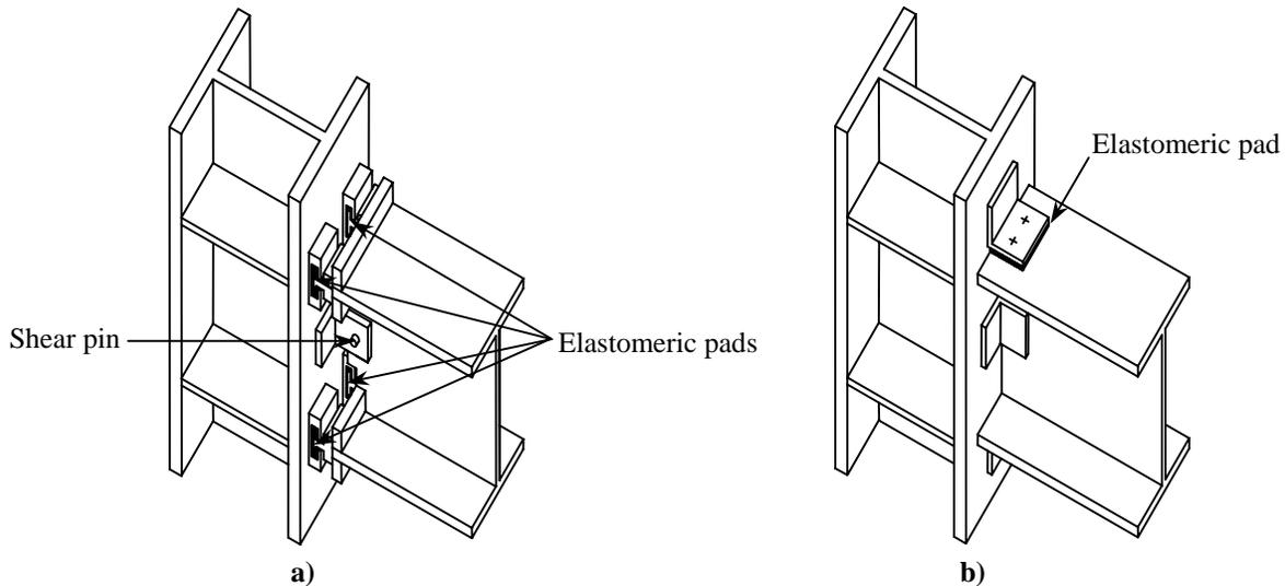
**Fig. 1 – 3D schemes of alternatives viscoelastic connections**
