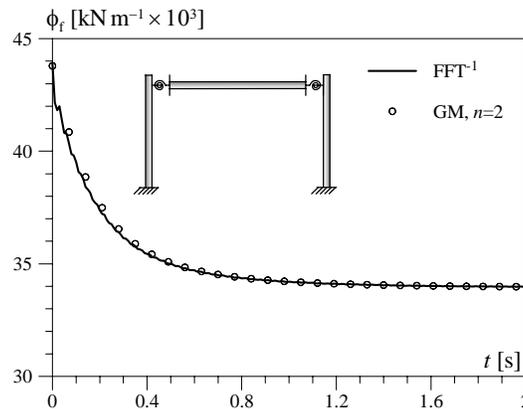
**Fig. 9 – Relaxation function of the portal frame with viscoelastic joints**
