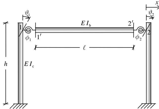
Fig. 7 – Single-story single-bay portal frame with viscoelastic beam-to-column connections
