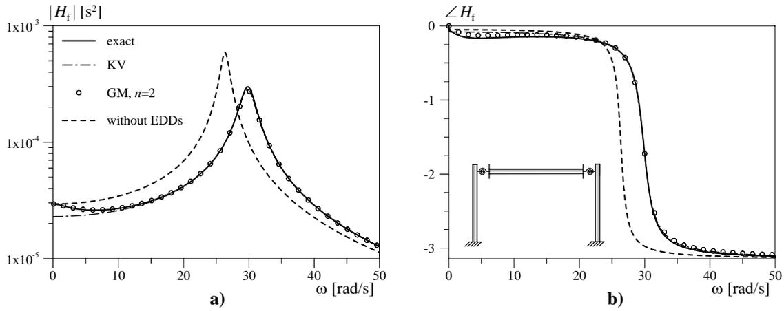
**Fig. 10 – Frequency Response Function of the portal frame with viscoelastic joints: a) modulus; b) argument**
