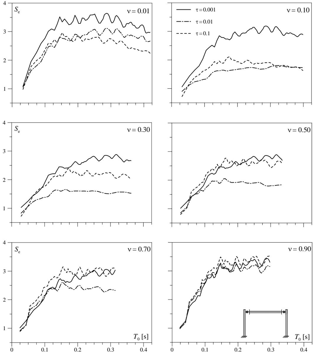
**Fig. 12 – Response spectra of a SDof frame with viscoelastic joints consistent with the design elastic spectrum for rigid soils given by the Italian seismic code**
