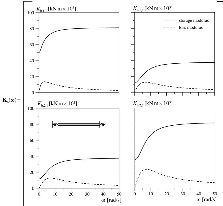
Fig. 6 – Dynamic stiffness matrix of the beam with viscoelastic hinges
