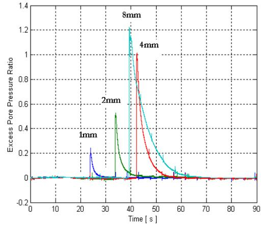
**Figure 5. Variation of excess pore pressure and pore pressure ratio with time**
