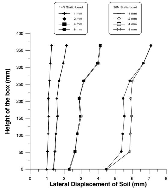
**Figure 7. Lateral soil displacement with height of the box for rigid pile wall**
