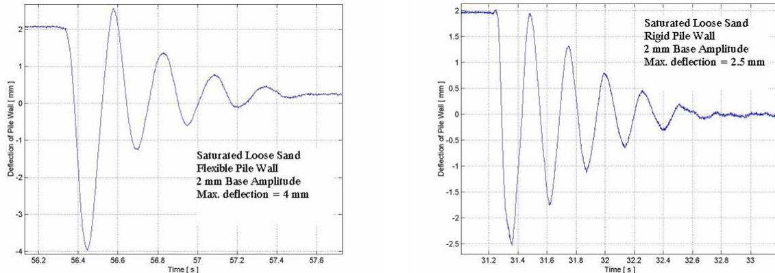
**Figure 8. Variation of deflection of the flexible and rigid pile walls with time in saturated loose sand with 2 mm base amplitude**
