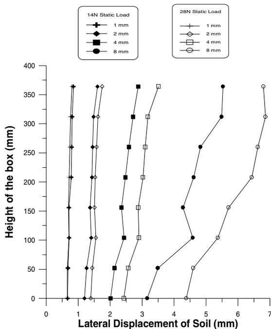
**Figure 2. Lateral soil displacement with height of the box for flexible pile wall**
