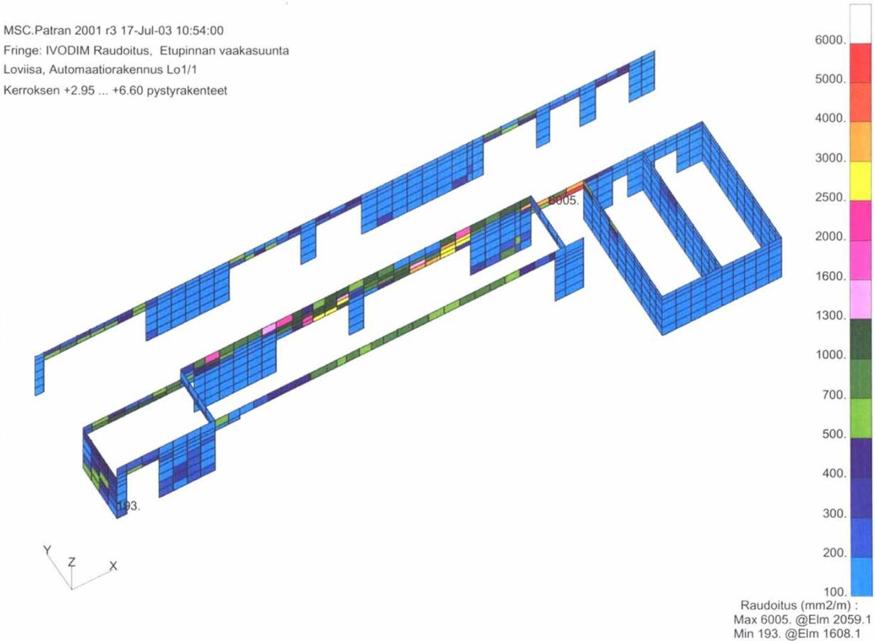
Figure 6 The horizontal reinforcement in front surfaces for storey +2.95 ... +6.60 in (mm<sup>2</sup>/m)
