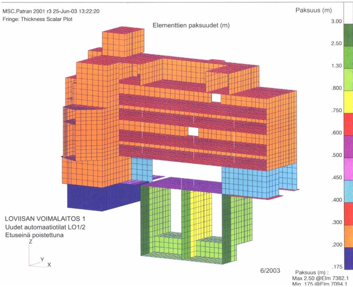
Figure 3 The 3D – structural model of building Lo1/2
