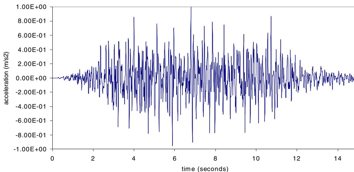
Figure 1 The x- component of simulated acceleration time history according to YVL 2.6.
