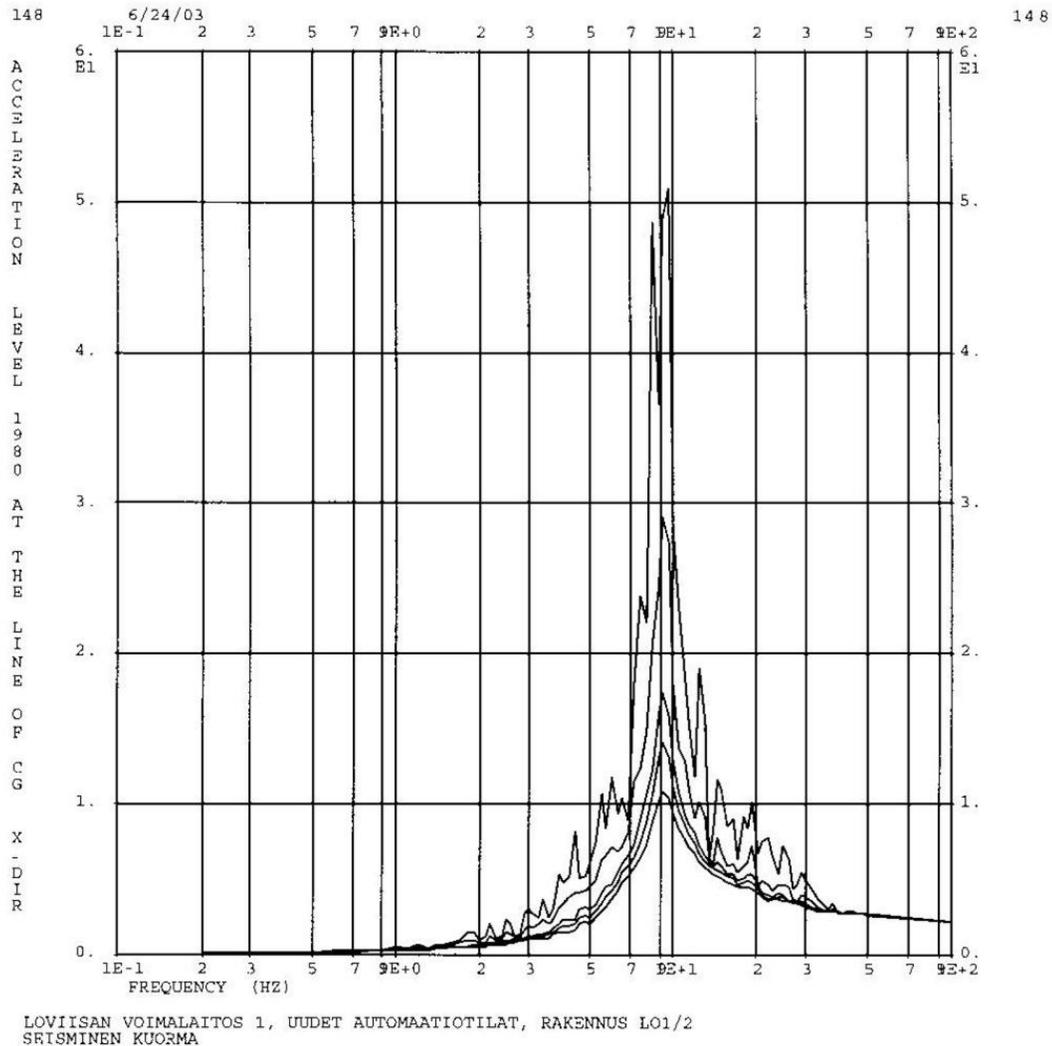
Figure 5 The floor response spectra at elevation +19.80 in X-direction for automation building Lo 1/2
