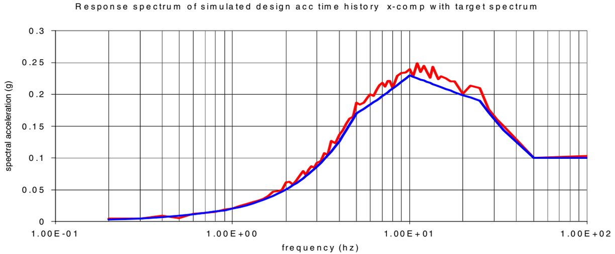
Figure 2 Response spectrum of simulated design acc time history x-comp with target spectrum
