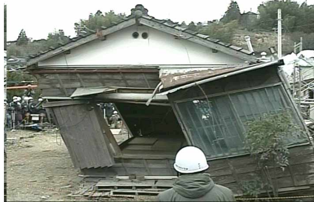
Figure 3 Pull Down Test of Aged Wood House
