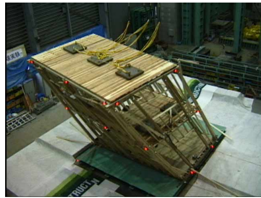
Figure 6 Collapse Test by Middle Size Shaking Table
