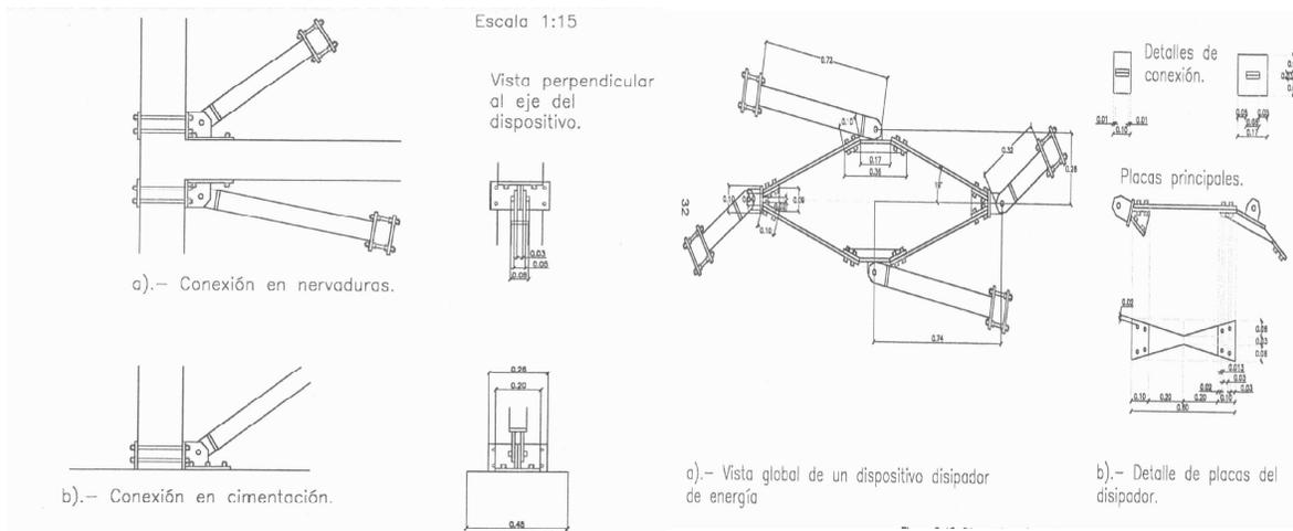
Figure 5. Foundation connection details
