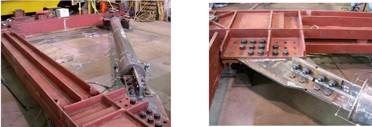
**Figure 2: Brace specimen in the test frame.**
