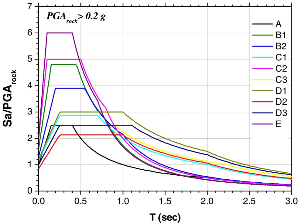
Figure 5. Proposed acceleration response spectra for each site category of table 1 and two levels of expected intensity ( $PGA_{rock} < 0.2g$  and  $PGA_{rock} > 0.2g$ ) normalized with respect to the maximum acceleration at ‘rock’ site conditions ( $PGA_{rock}$ ).
