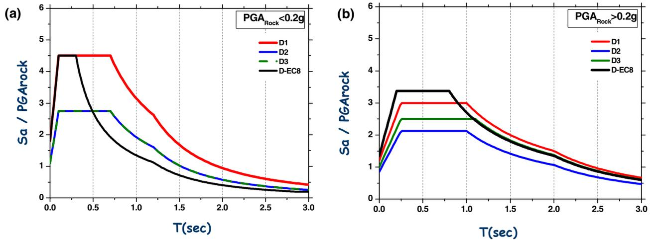
**Figure 8. Acceleration response spectra for D soil sites: Comparison of proposed values with those provided by EC8 for (a)  $PGA_{rock} < 0.2g$  and (b)  $PGA_{rock} > 0.2g$**
