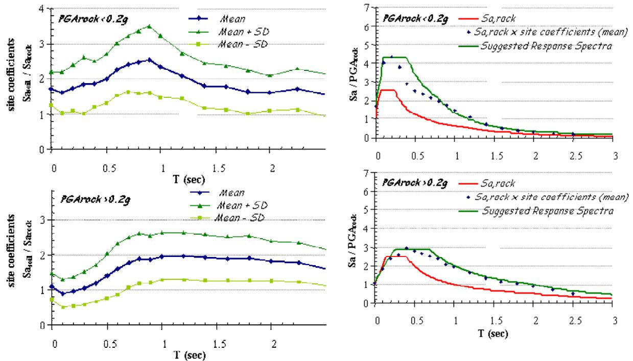
Figure 4. Site category C1: (a) Spectral amplification factors – Results of theoretical seismic response, (b) Proposed acceleration response spectra.
