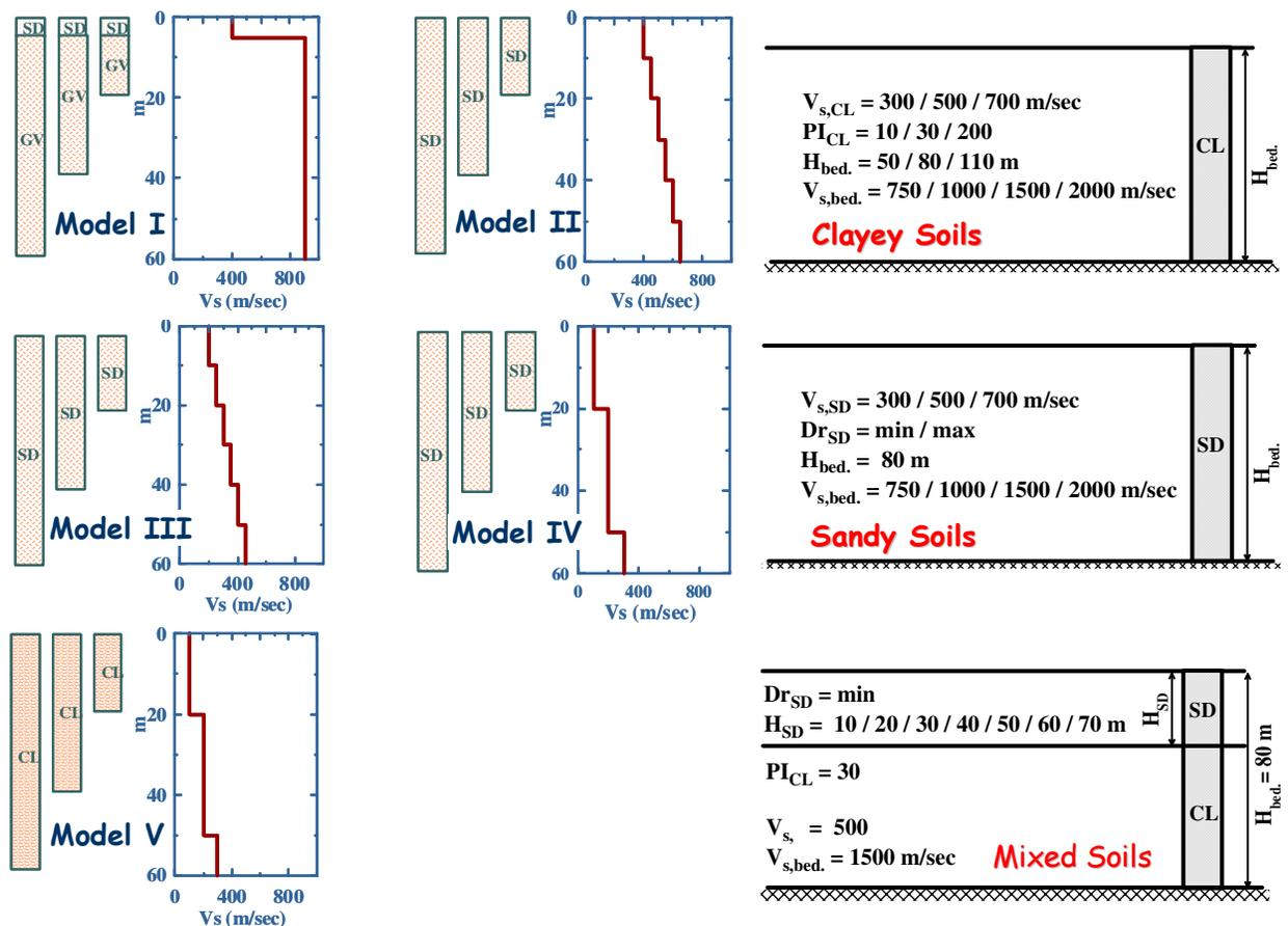
**Figure 2. (a) Soil models according to EC8 classes, (b) Clayey, sandy and mixed soil models used in theoretical analyses.**
