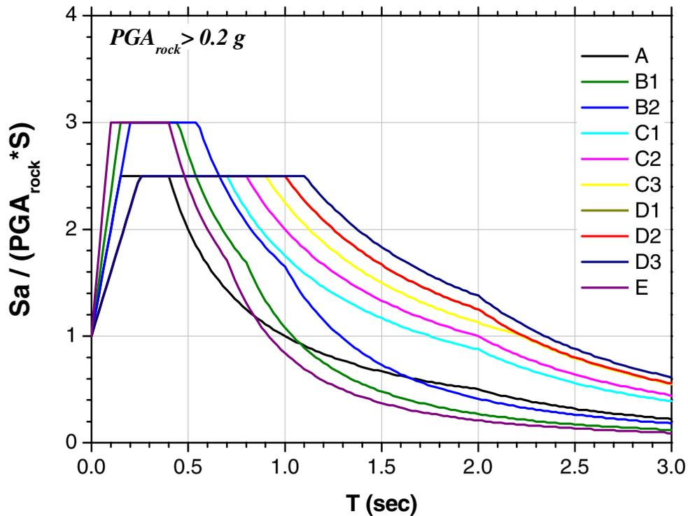
Figure 6. Normalized acceleration response spectra for each site category of Table 1 and two levels of earthquake intensity ( $PGA_{rock} < 0.2g$  and  $PGA_{rock} > 0.2g$ ); normalized with respect to the maximum ground acceleration ( $PGA_{rock} * S$ ).
