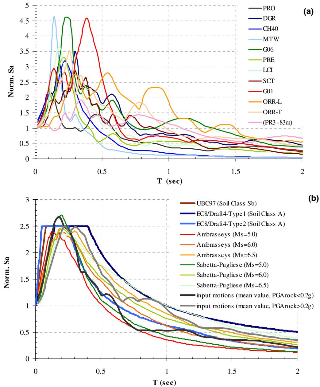
**Figure 3. (a) Normalized acceleration response spectra of the 12 selected seismic excitations used in theoretical analyses, (b) acceleration response spectra at ‘rock’ sites: comparison of values proposed by seismic codes and empirical attenuation relationships.**
