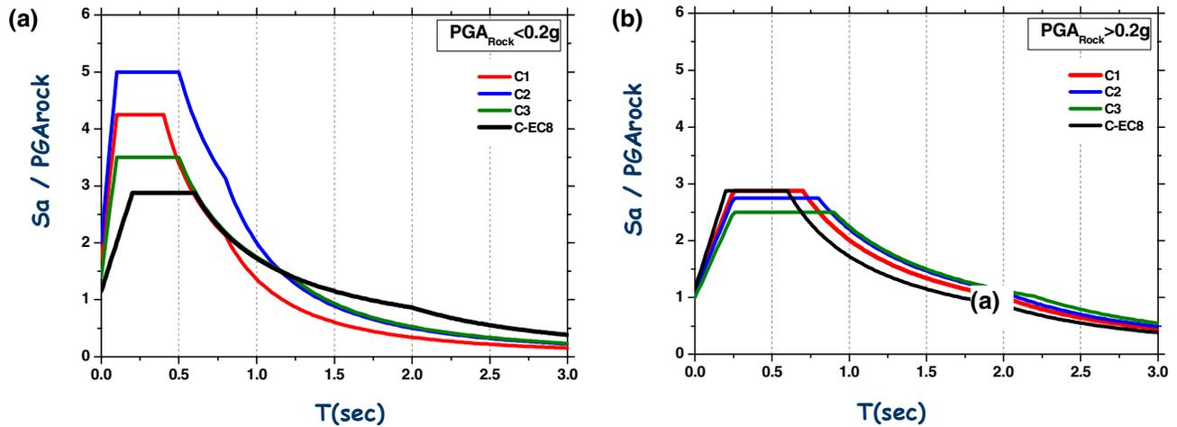
**Figure 7. Acceleration response spectra for C soil sites: Comparison of proposed values with those provided by EC8 for (a)  $PGA_{rock} < 0.2g$  and (b)  $PGA_{rock} > 0.2g$**
