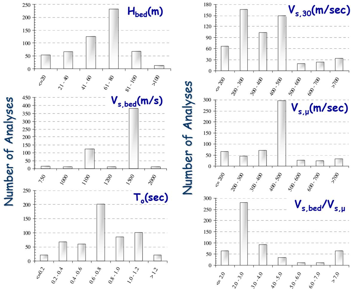
**Figure 1. Soil models used in the theoretical analyses: Variation of (a) depth of bedrock, (b)  $V_s$  of bedrock ( $V_{s,bed}$ ), (c) fundamental period of soil deposit, (d) fluctuation of mean value of  $V_{s,30}$ , (e) mean shear wave velocity of soil deposit  $V_{s,m}$  and (f) impedance ratio  $V_{s,bed}/V_{s,m}$ .**
