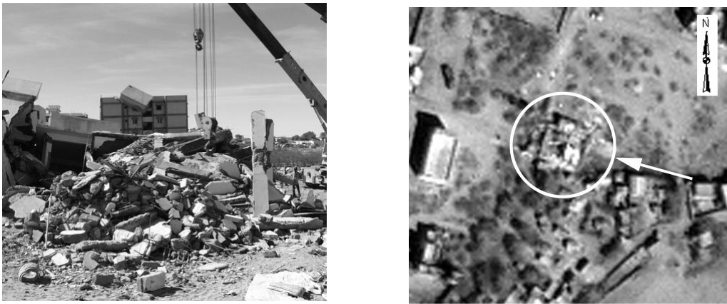
Figure 1. Photo (left) and satellite image (right) of a collapsed single building in the north of Bhuj. The remains of the building are visible in the satellite image. The white arrow in the satellite image shows the look angle of the photo.
