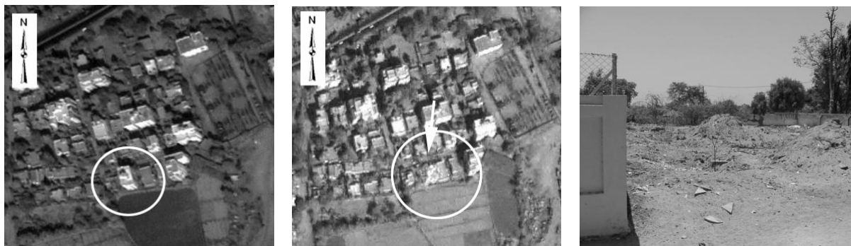
Figure 3. Example of an image of a collapsed building. Left: pre-earthquake image; middle: post-earthquake image; right: ground photograph of the same site 15 months after the earthquake. The ground photograph was taken by the authors.
