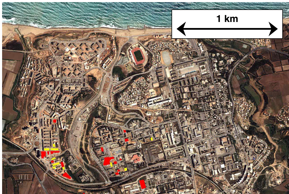
Figure 8. Collapsed (red) and heavily damaged (yellow) structures identified from visual examination of pre- and post-earthquake images.
