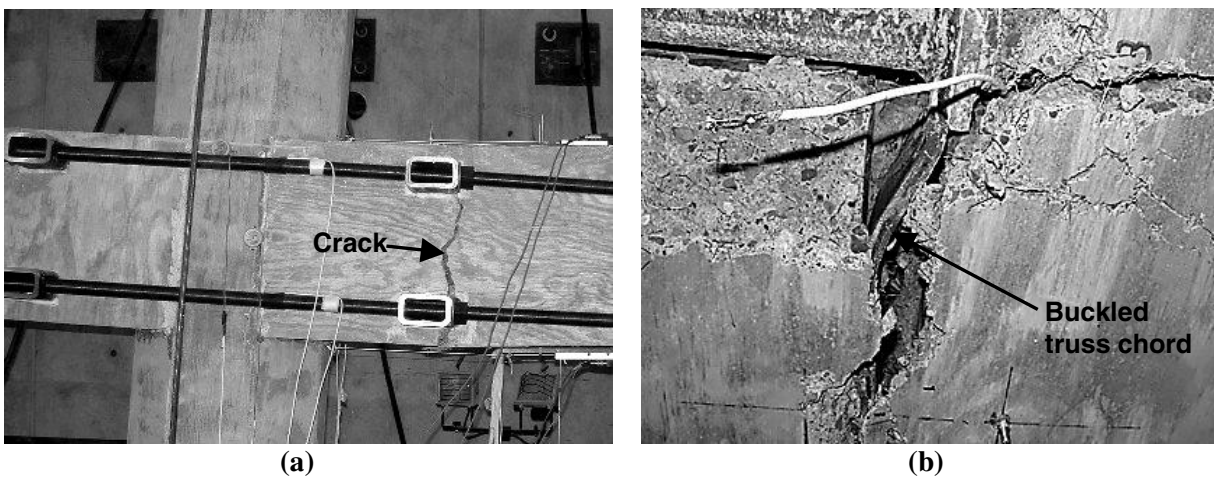
Figure 7: Damage in Specimen 1 at 5.0% drift (a) single major crack at transverse tube face, (b) buckling of truss chord
