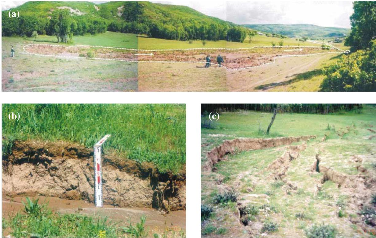
Figure 5. (a) A general view of the lateral spreading and flow at Hanoçayırı, (b) vertical drops and (c) separations due to lateral spreading.
