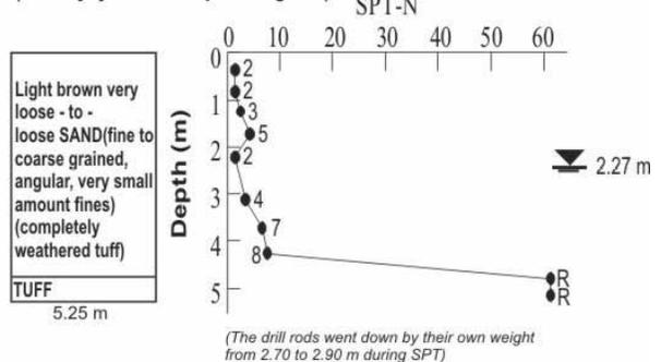
(R: Rejected; ie. N>50 between the interval of 15-30 cm of SPT test)
