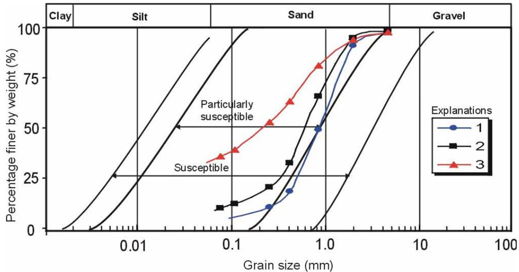
Figure 6. Grain size distribution of the ejected (samples 1 and 2) and flowed (sample 3) material.
