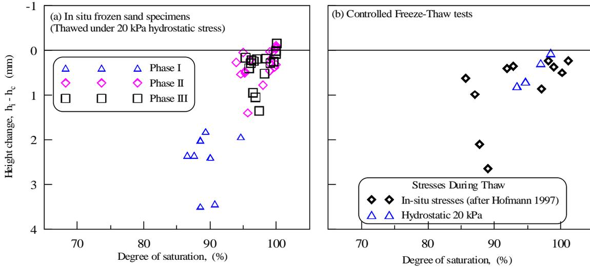
Figure 1: Height change during thaw and consolidation in Mildred Lake sand
