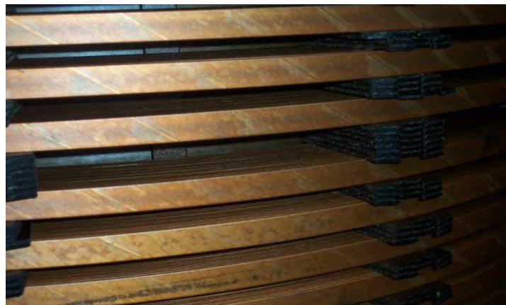
Figure 5. Key spacers separating different layers of winding.
