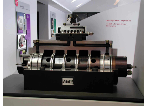
Fig. 7: MTS 10,000 liter/min High Performance Servo-valve
