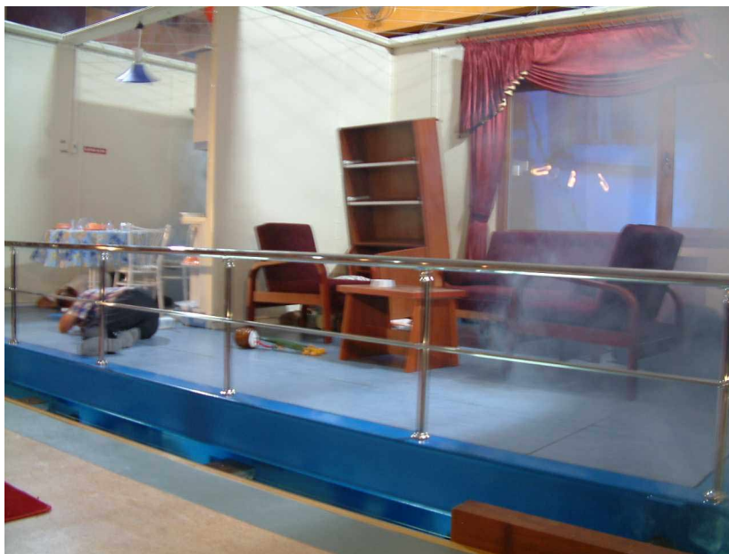
Fig. 5- The “mobile stage” in motion. Note the person lying on the stage-floor on the left for protection, the tilted bookshelves (to be brought back to the upright position automatically, after the scenario ended), the fallen flower-pot near the center, the generated smoke and the moving video image (seen through the window) on the right.
