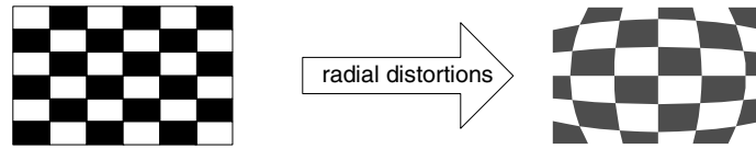
Figure 2. Effect of radial distortions with real lenses, barrel distortions.
