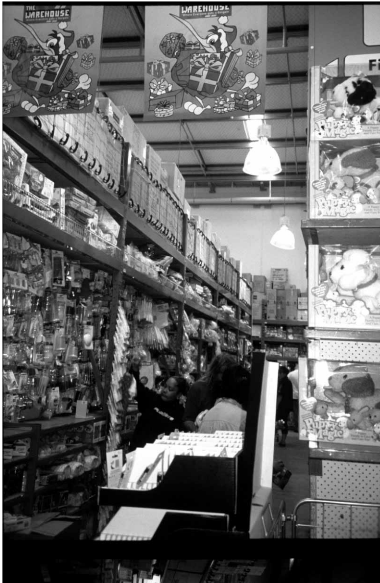
Figure 8: Retail shop showing a good rope system installed on higher shelves to restrain goods from falling, but some of the highest boxes are above the restraints (from Dowrick [7]).
