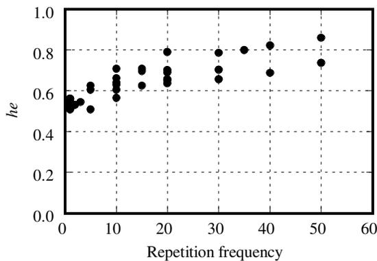
Figure 13 The relation of repetition frequency to equivalent damping coefficient
