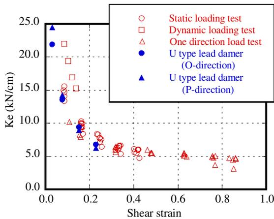
Figure 11 The relation of shear strain to equivalent spring coefficient
