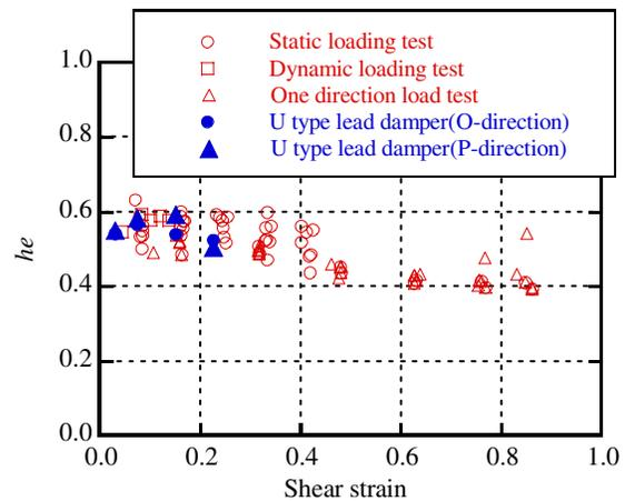
Figure 12 The relation of shear strain to equivalent damping coefficient
