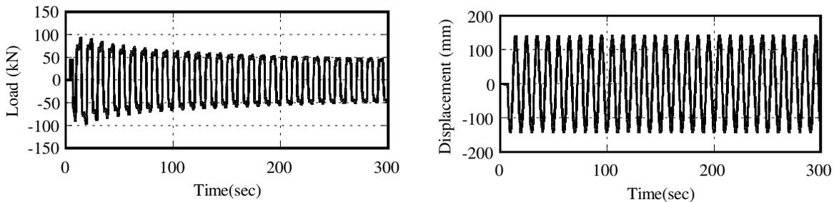
Figure 7 Results of fatigue test (time history)
