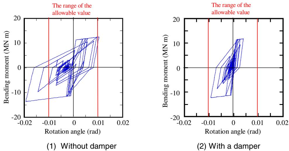
Figure 16 The relation of bending moment to rotation angle
