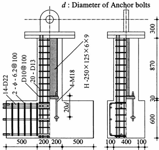
Fig. 1 Test specimen V4B (Unit : mm)
