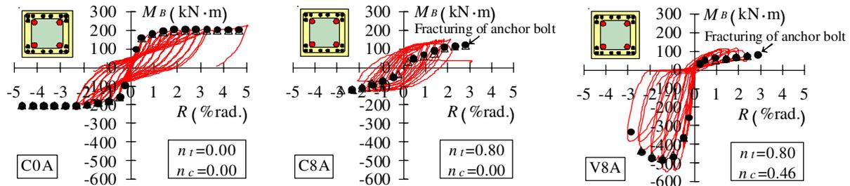
Fig. 12 Relationships of bending moment and deflection angle
