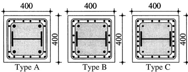
Fig. 2 Section of column (Unit : mm)
