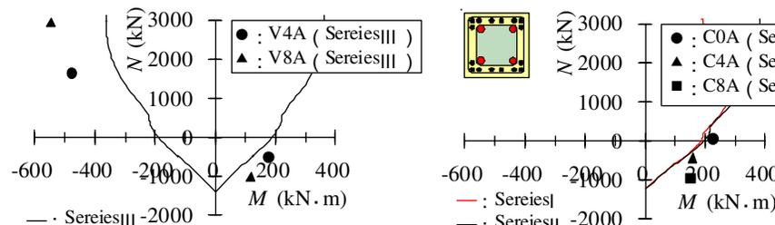
Fig. 5 Relationships of axial force and ultimate bending moment
