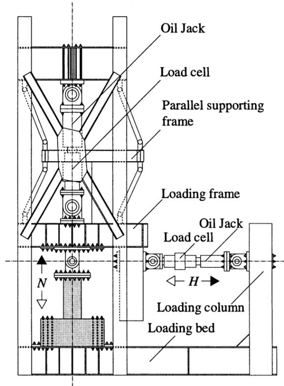
Fig. 3 Test setup system
