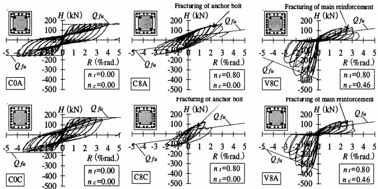
Fig. 4 Relationships of lateral load and deflection angle
