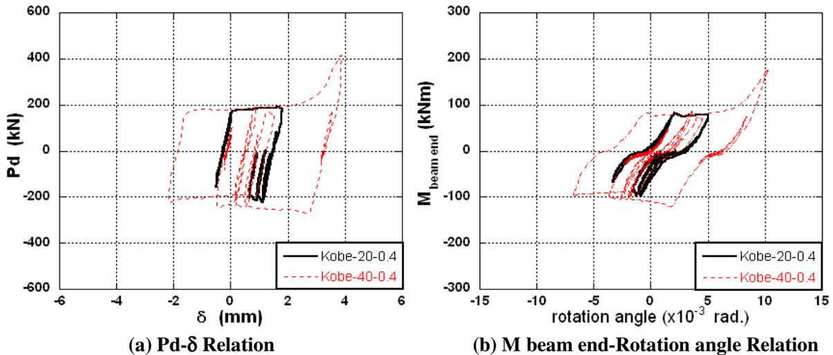
Fig. 10 Experimental Result of PL2 Specimen under Random Excitations (Kobe-20, 40-0.4)
