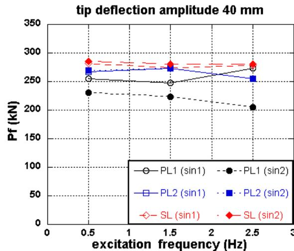
Fig. 12 Effect of Excitation Frequency on Resisting force (Tip Deflection Amp. 40 mm)
