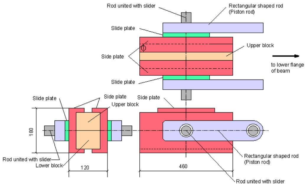
**Fig. 1 Outer View of Lead Damper (unit: mm)**
