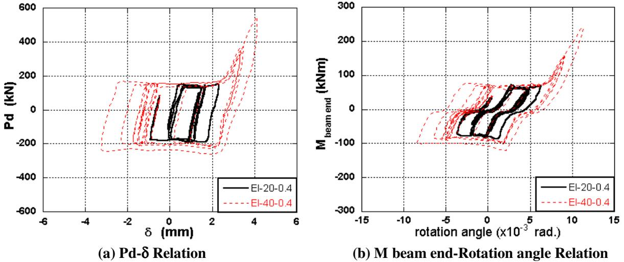
Fig. 9 Experimental Result of PL1 Specimen under Random Excitations (EI-20, 40-0.4)
