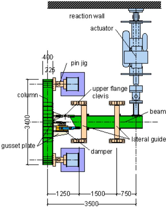
**Fig.4 Test Set-up (unit: mm)**
