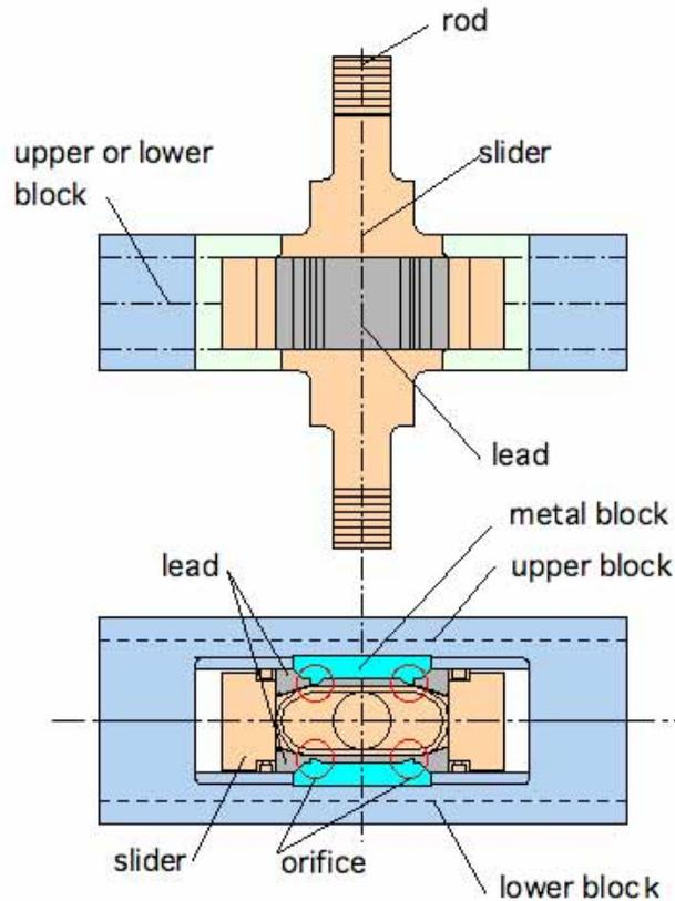
**Fig.2 Cross Section of Lead Damper**
