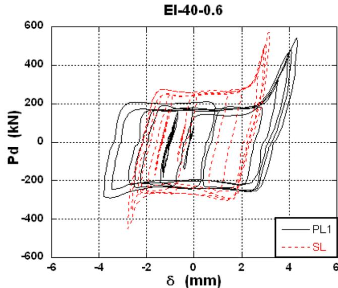
**Fig. 14 Comparison of Hysteresis loops between PL and SL Specimens**
