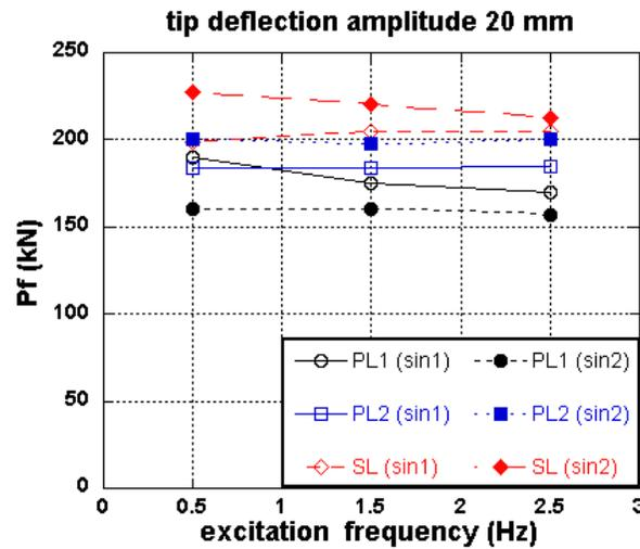
Fig. 11 Effect of Excitation Frequency on Resisting force (Tip Deflection Amp. 20 mm)
