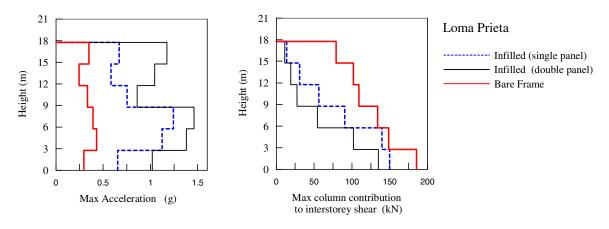
Figure 15 Time-history analyses on the 6-storey frames (case-study):maximum floor acceleration and interstorey shear column contribution; comparison between bare and non-uniformely infilled frames response (Loma Prieta Record)
