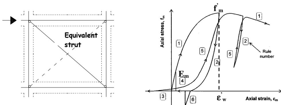
Figure 3 Equivalent strut model for masonry infills and hysteresis rule adopted (Crisafulli [17])
