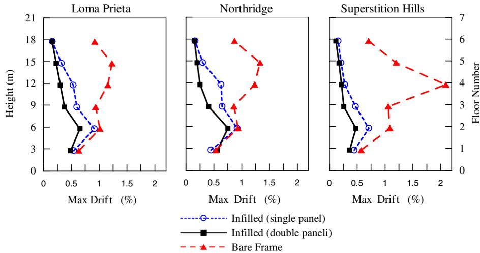
**Figure 14 Time-history analysis on the 6-storey frames (case-study): maximum interstorey drift; comparison between bare and uniformly infilled frames response**
