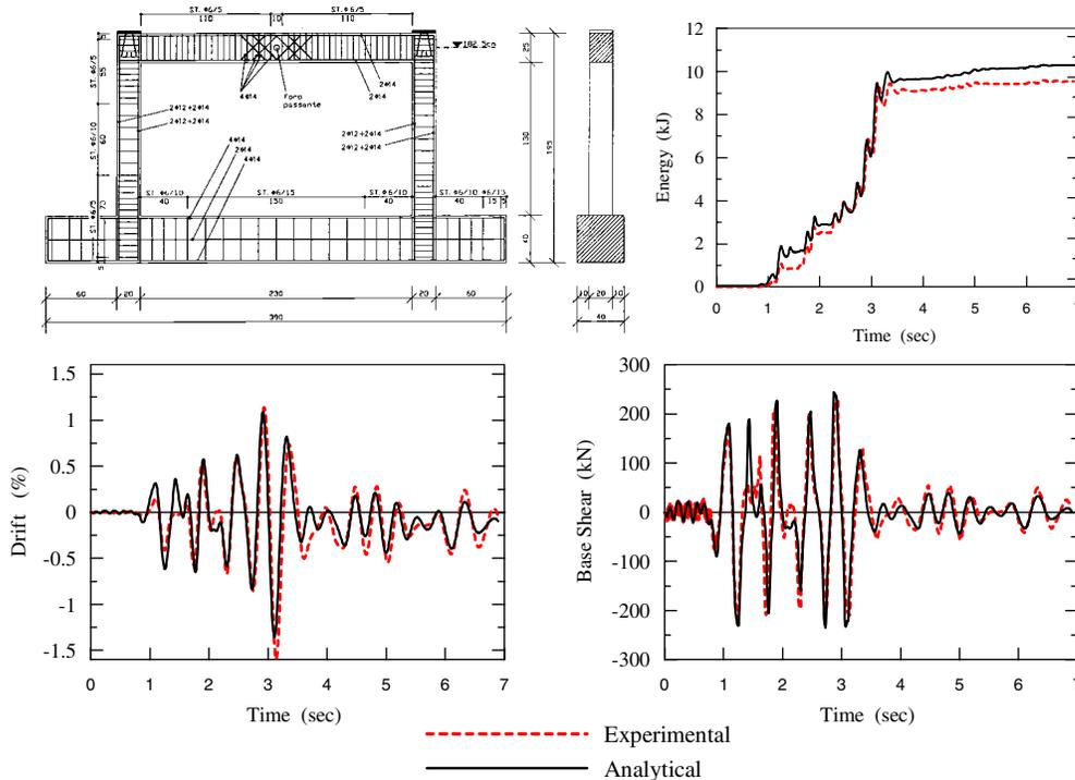
**Figure 5 Analytical-experimental comparison on pseudo-dynamic tests on portal frame with infills (Specimen L2, University of L’Aquila [19])**
