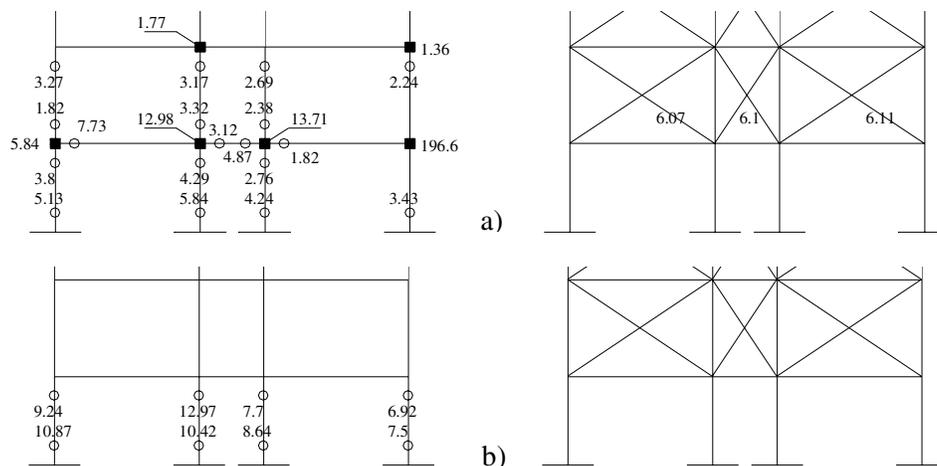
**Figure 12 Non-uniformly infilled frame damage mechanism (plastic hinges, shear hinges, ductility demand) at 1% top drift: a) Non-linear modelling of joints, b) Elastic modelling of joints**
