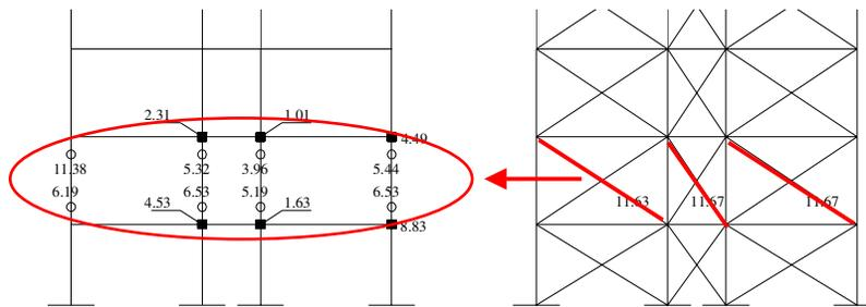
**Figure 11 Uniformly infilled frame damage mechanism (plastic hinges, shear hinges, ductility demand) at 1% top drift**
