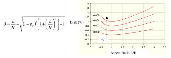
Figure 8 Relationship between strut axial strain Ew, interstorey drift and aspect ratio L/H
