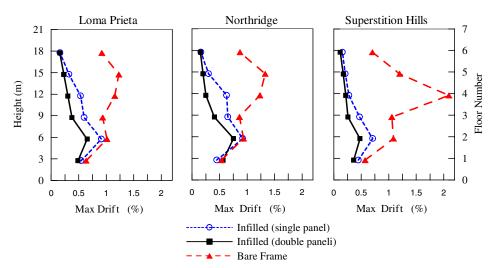
Figure 14 Time-history analysis on the 6-storey frames (case-study): maximum interstorey drift; comparison between bare and uniformly infilled frames response
