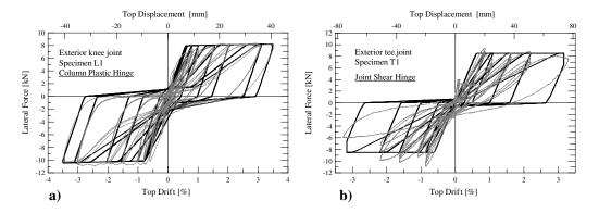
Figure 4 Analytical-experimental comparison on cyclic tests on beam-column subassemblies a) flexural plastic hinge; b) joint shear hinge (University of Pavia, [1])
