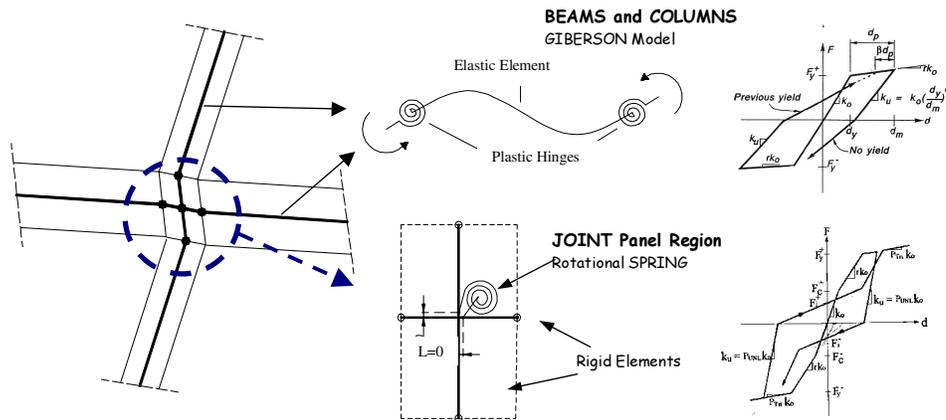
**Figure 2 Modelling of structural elements: beams, columns (plastic hinges) and joint panel region (shear hinge)**
