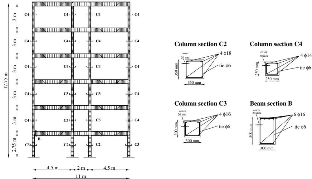
**Figure 9 Geometric and mechanical characteristics of the 6-storey frame (case-study)**
