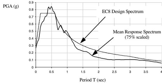
**Figure 13 Characteristics of the selected Earthquake Records; mean elastic response spectrum and compatibility with EC8 design spectrum (PGA 0.3g)**
