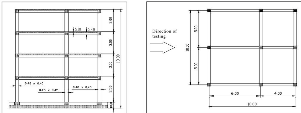
**Figure 6 Four-Storey Frame Building tested at ELSA (JRC, Ispra, Italy [24]): elevation and plan view**
