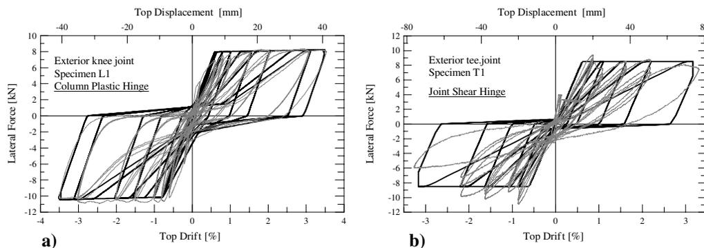
**Figure 4 Analytical-experimental comparison on cyclic tests on beam-column subassemblies**
