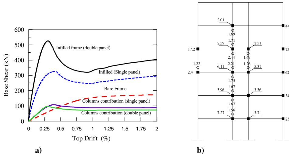
**Figure 10 Pushover analyses on the 6-storey frames: a) Comparison of the monotonic response; b) Bare frame damage mechanism (plastic hinges, shear hinges, ductility demand) at 1% top drift**
