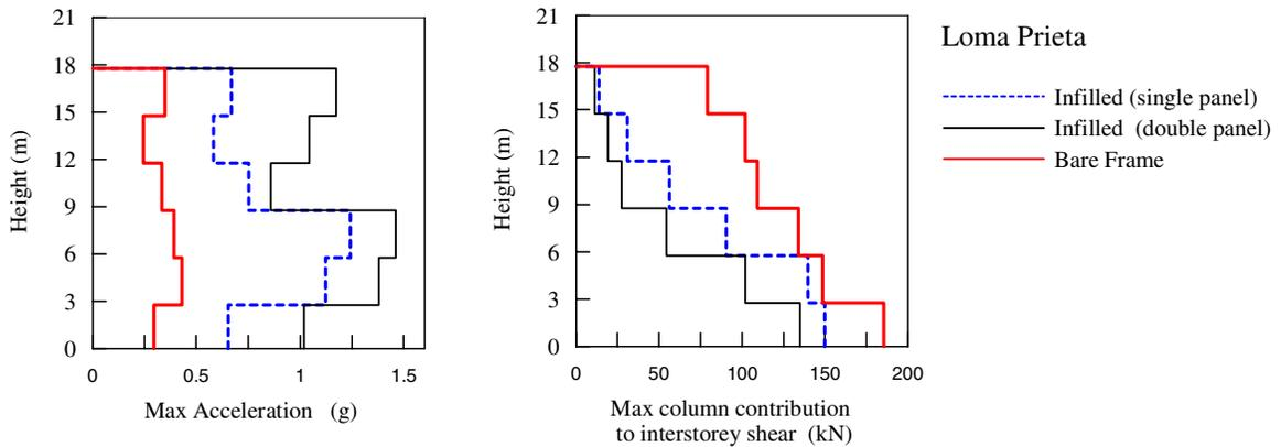
**Figure 15 Time-history analyses on the 6-storey frames (case-study): maximum floor acceleration and interstorey shear column contribution; comparison between bare and non-uniformly infilled frames response (Loma Prieta Record)**
