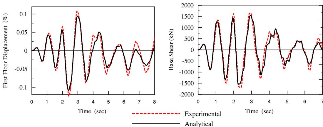
**Figure 7 Analytical-experimental comparison of the pseudo-dynamic response on a four-storey infilled frame (ELSA Laboratory, Ispra JRC [24]): first floor and base shear time-history**
