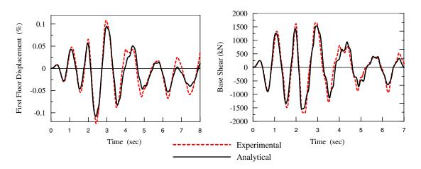
Figure 7 Analytical-experimental comparison of the pseudo-dynamic response on a four-storey infilled frame (ELSA Laboratory, Ispra JRC [24]): first floor and base shear time-history
