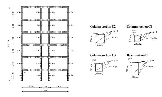
Figure 9 Geometric and mechanical characteristics of the 6-storey frame (case-study)
