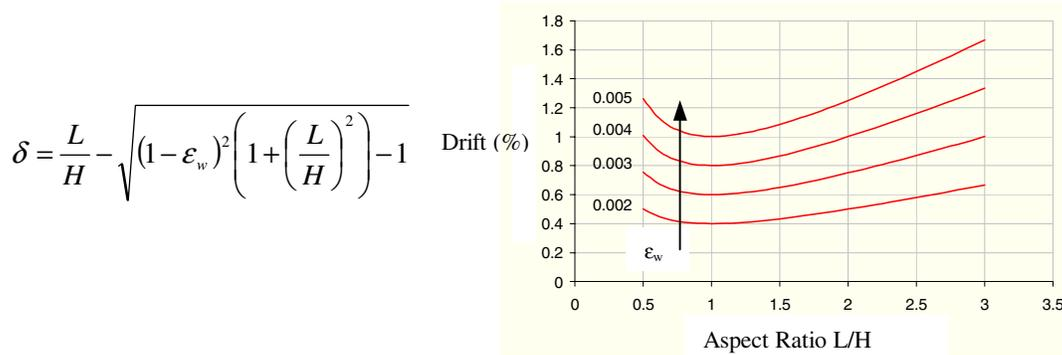
**Figure 8 Relationship between strut axial strain  $\epsilon_w$ , interstorey drift and aspect ratio  $L/H$**
