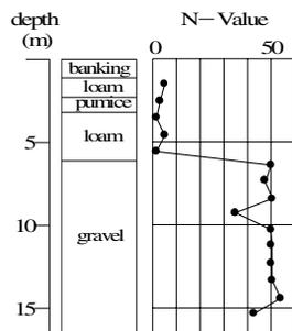
Fig.1 Soil profile where R/C bldg stand on
