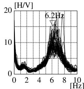
Fig.2 H/V spectral ratio of soil
