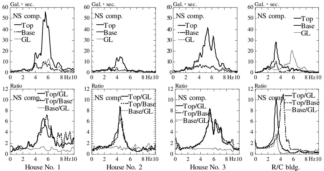
Fig.5 Fourier spectra and its ratios of Eq. No.23 of NS component
