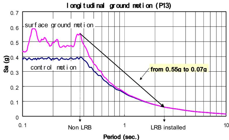
**Fig. 12 The effect of base isolation system.**
