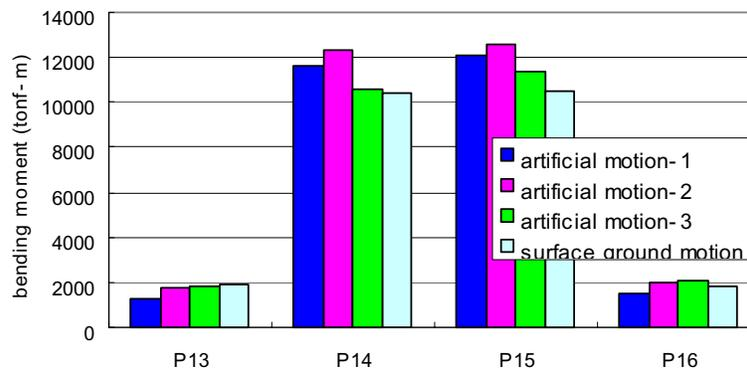
**Fig. 10 Member force of pier by longitudinal input motion.**
