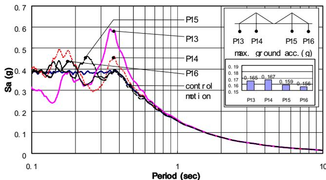
**Fig. 9 Comparison of response spectrum in transverse direction.**
