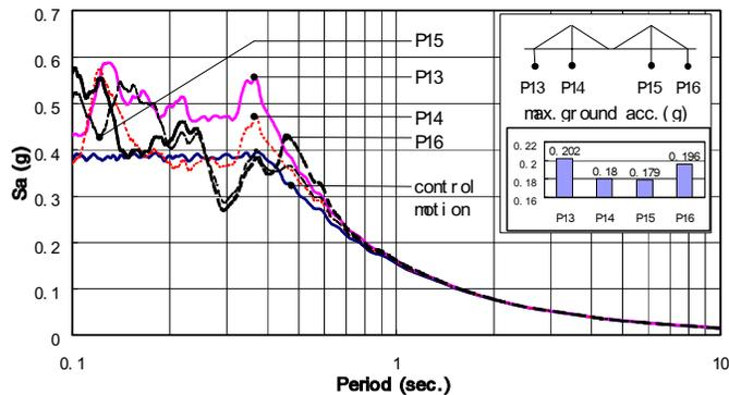
**Fig. 8 Comparison of response spectrum in longitudinal direction.**
