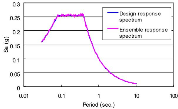
**Fig. 7 Acceleration response spectrum of averaged artificial motion.**
