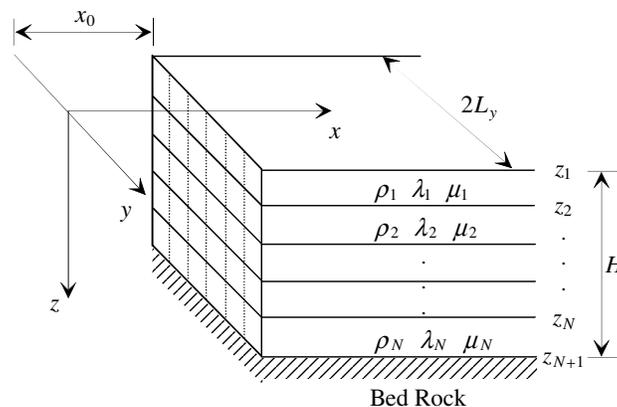
Fig. 1 Transmitting boundary located at  $x = x_0$ .
