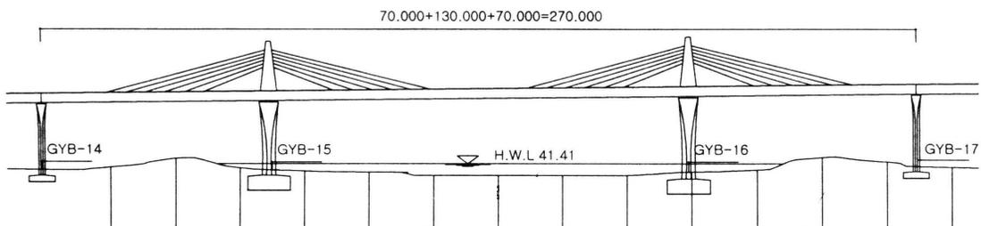
**Fig. 3** Three span extradossed bridge.
