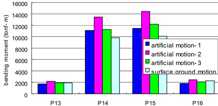
**Fig. 11 Member force of pier by transverse input motion.**
