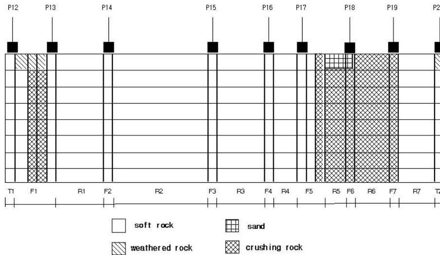
**Fig. 6 2-D hybrid modeling of the ground.**
