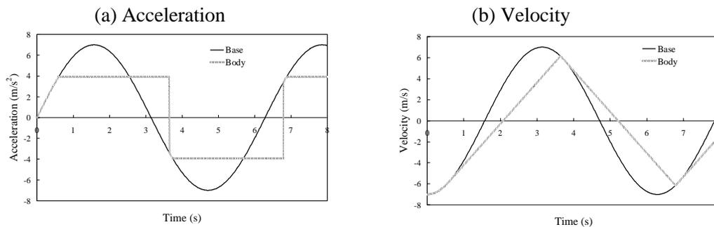
**FIGURE A1. ACCELERATION AND VELOCITY TIME HISTORIES OF THE BASE AND BODY**
