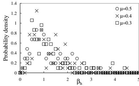
**FIGURE 4. EFFECTS OF THE VERTICAL GROUND MOTION ON THE SLIP DISPLACEMENT (EX. PHGA=9m/s<sup>2</sup>)**
