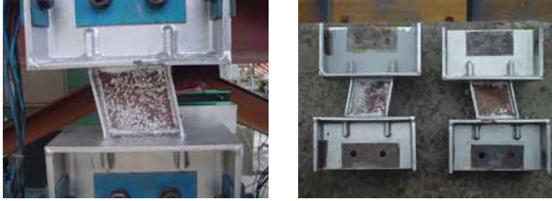
Photo 2 Hysteretic dampers after pseudo-dynamic response test
