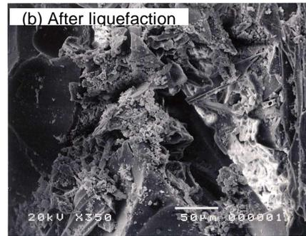
**Photographs 2 SEM of disturbed samples ( $\sigma_{30}'=98\text{kPa}$ )**
