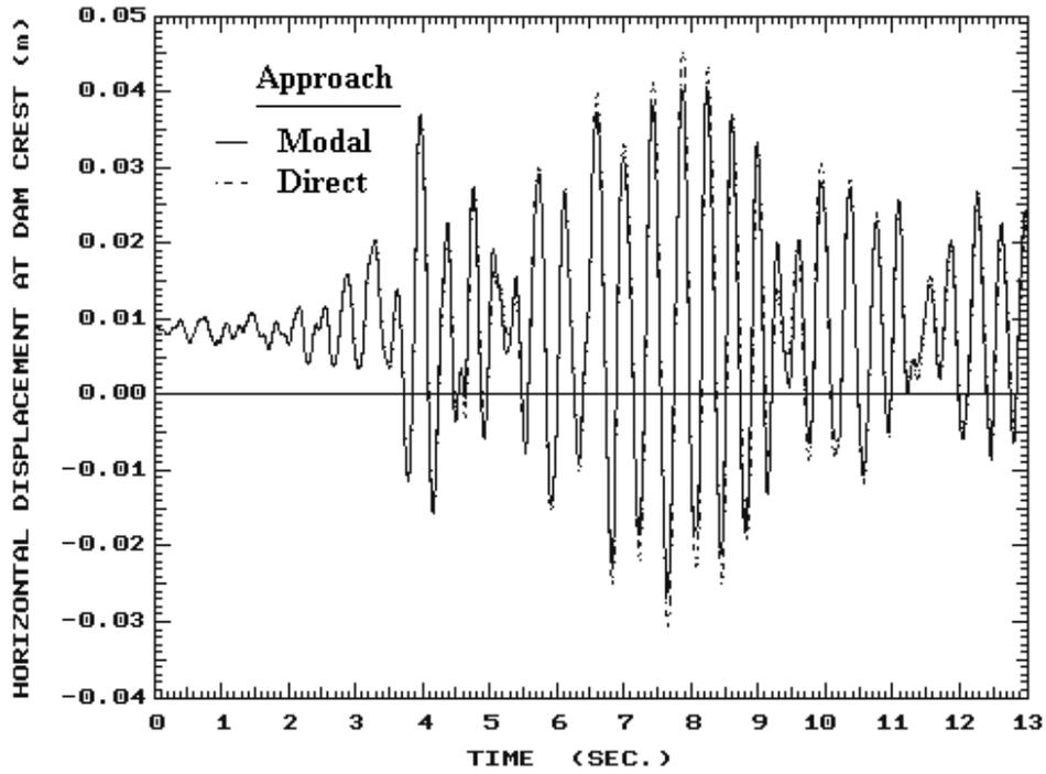
Figure 5. Comparison of displacement history at dam crest between the two approaches.
