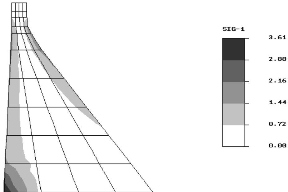
Figure 7. Envelope of maximum tensile principal stresses (MPa) when the number of modes utilized are doubled over the original case.
