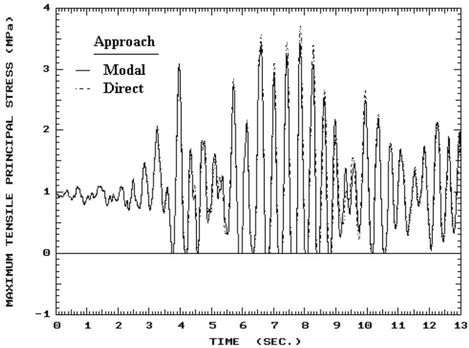
Figure 6. Comparison of maximum tensile stress history at dam heel between the two approaches.
