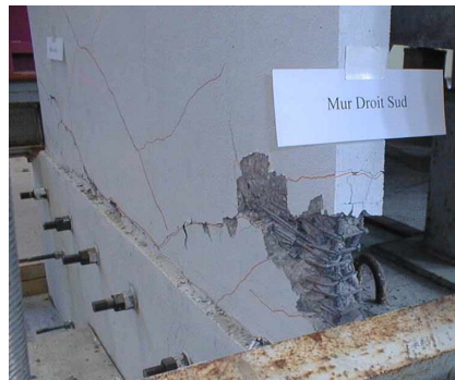
Figure 5. Damage to the free edge of the wall at the end of the test sequence (CAMUS 3)
