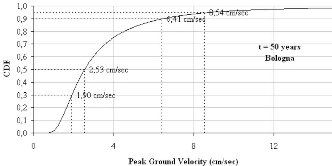
**Fig. 4. Cumulative Distribution Function (CDF) of the Peak Ground Velocity for the city of Bologna (P.za Maggiore) for an observation time  $t = 50$  years.**
