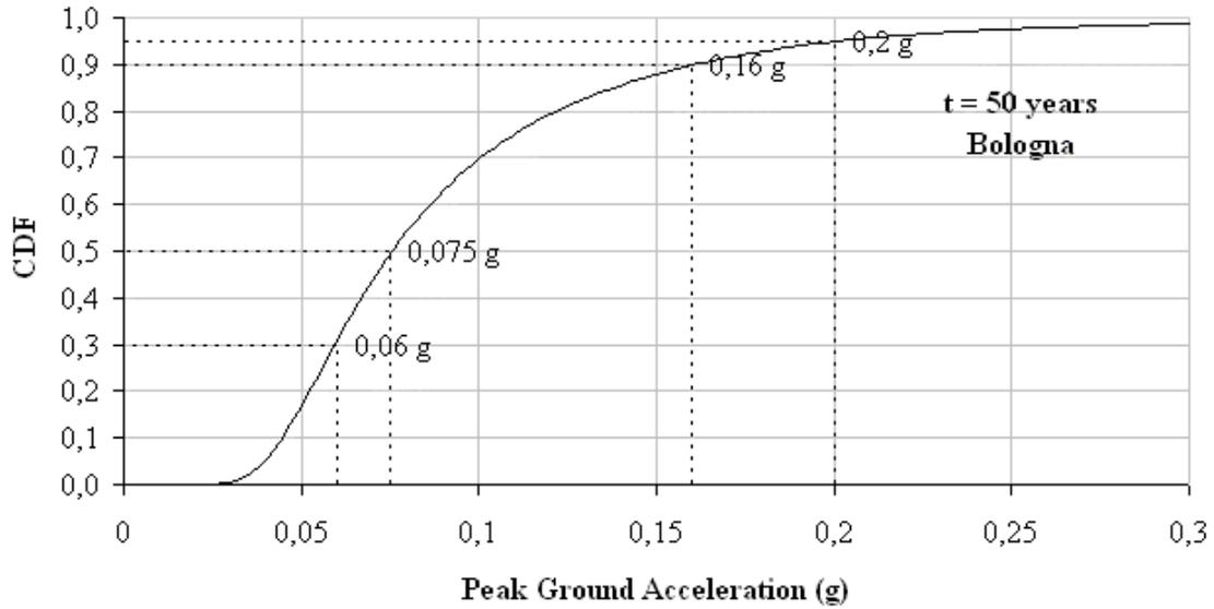
**Fig. 3. Cumulative Distribution Function (CDF) of the Peak Ground Acceleration for the city of Bologna (P.za Maggiore) for an observation time  $t = 50$  years.**
