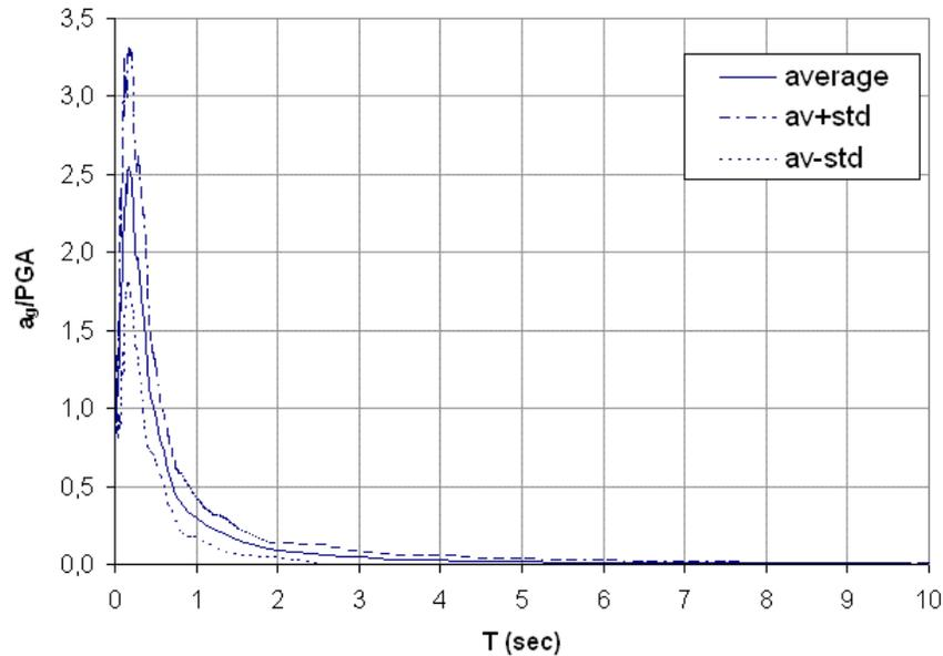
**Fig. 6: response spectra (average, average +/- one standard deviation) for “bouquet B” of earthquake records (vectorial Intensity Measure)**
