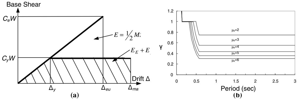
**Figure 4:** (a) Energy input in elastic and inelastic systems, (b) Energy modification factors against period
