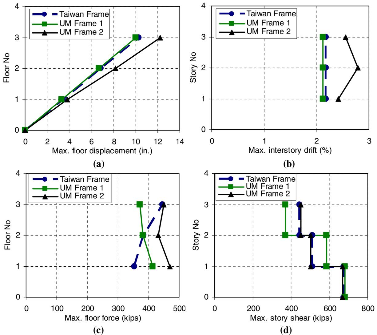
**Figure 9:** Dynamic response parameters of three frames for Taiwan site
