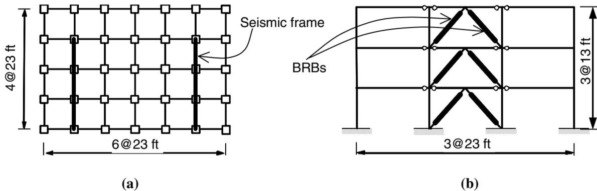
**Figure 1:** (a) Layout of the prototype building, (b) View of the test frame
