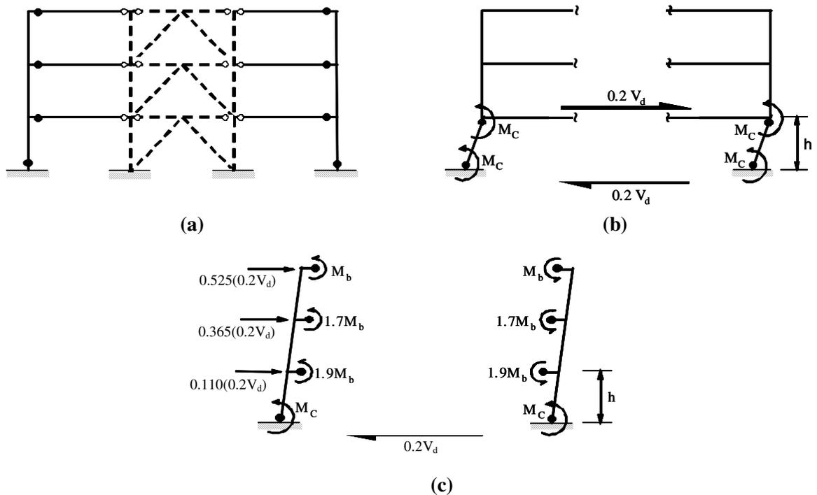
**Figure 5:** (a) Moment frame yield mechanism, (b) Minimum column strength from story mechanism, and (c) Moment demands on beams
