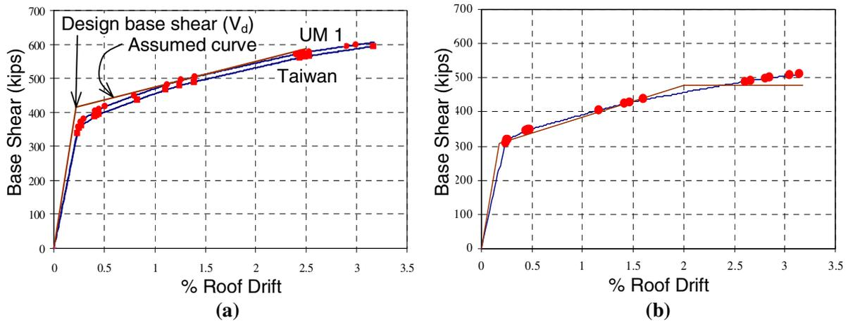
**Figure 7:** (a) Push-over curves for Taiwan Frame and UM Frame 1, and (b) Push-over curve for UM Frame 2
