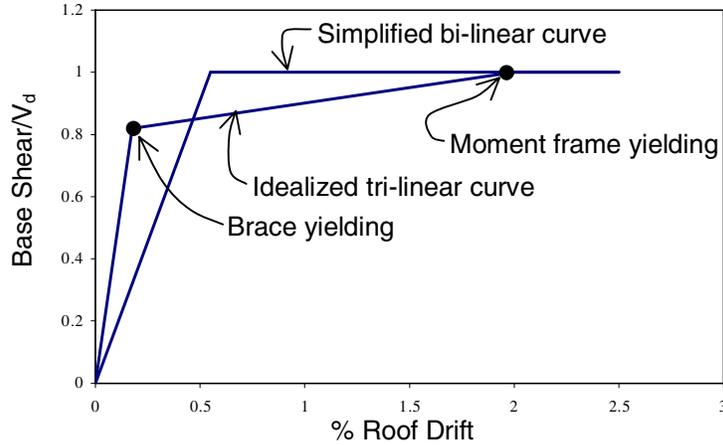
**Figure 3:** Idealized frame responses for *Collapse Prevention* criterion
