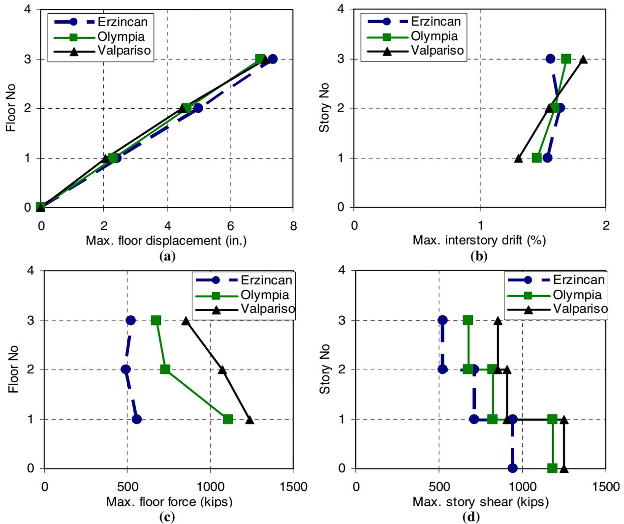
**Figure 10:** Dynamic response parameters of frame UM-US for three Seattle ground motions
