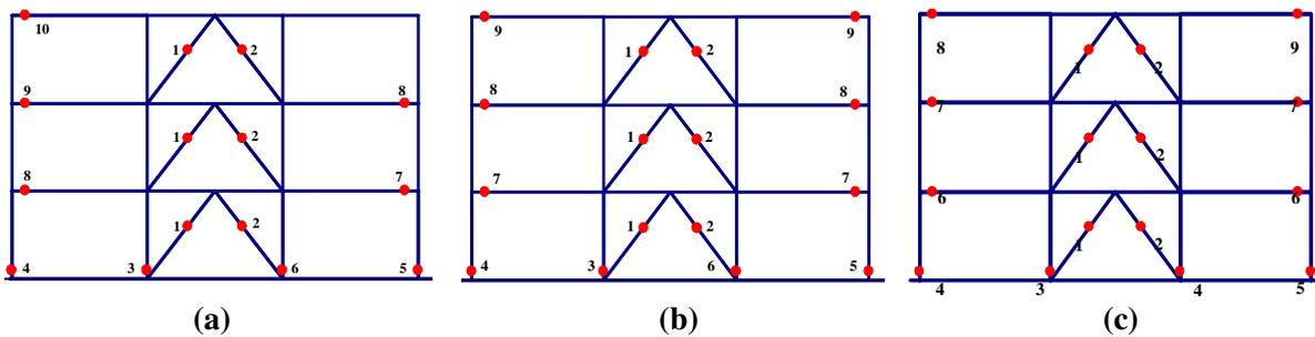
**Figure 8:** Locations and sequence of yielding - (a) Taiwan Frame, (b) UM Frame 1, and (c) UM Frame 2
