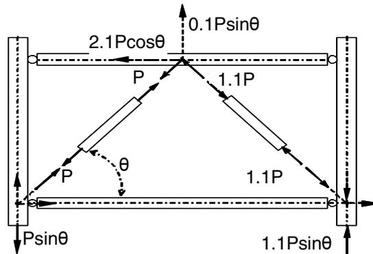
**Figure 6:** Forces in braced frame after yielding
