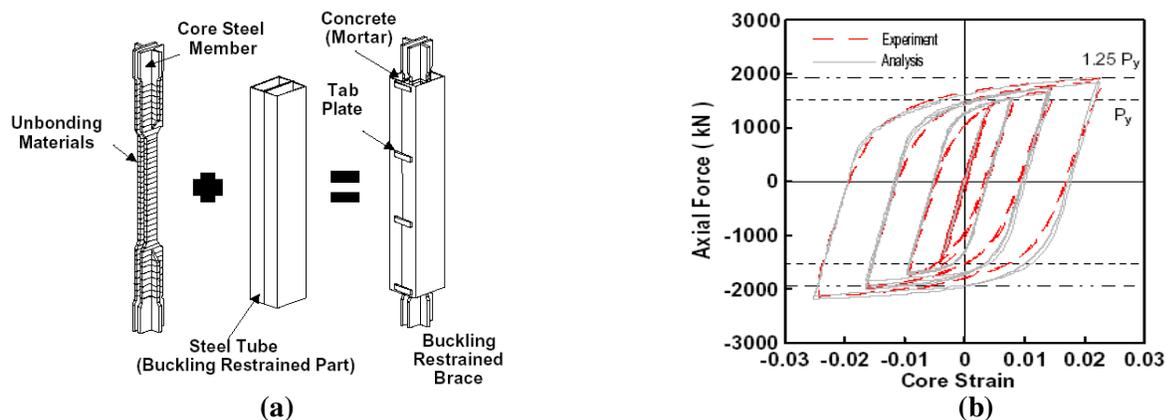
**Figure 2:** (a) Configuration of the BRB adopted, and (b) Typical load-displacement behavior of a BRB (From Tsai [1])
