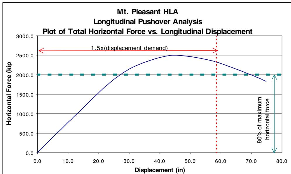
**Figure 9 – Force vs. Displacement Curve at Deck Level for Mt. Pleasant High Level Approach**
