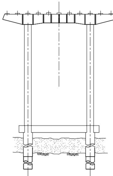
**Figure 4 – Typical Concrete Pier**
