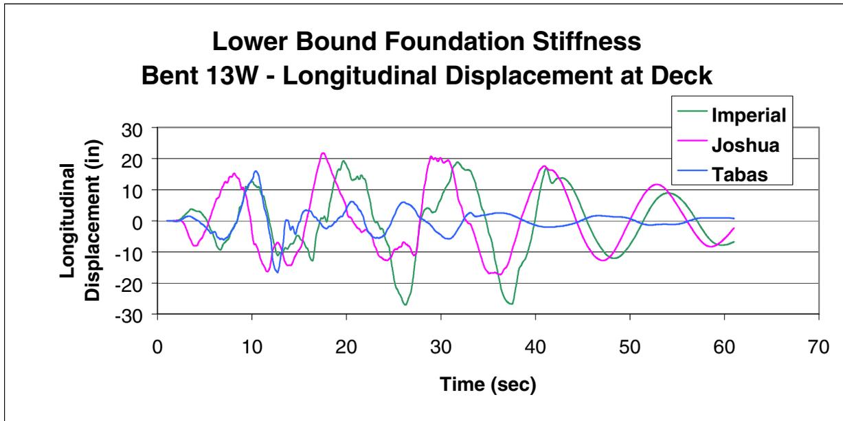
Figure 10 – Longitudinal Displacement Response Time Histories at Deck Level for Charleston High Level Approach
