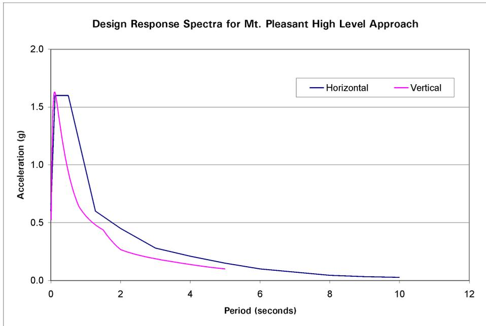
**Figure 2 – Design Response Spectra at Foundation for Mt. Pleasant High Level Approach**
