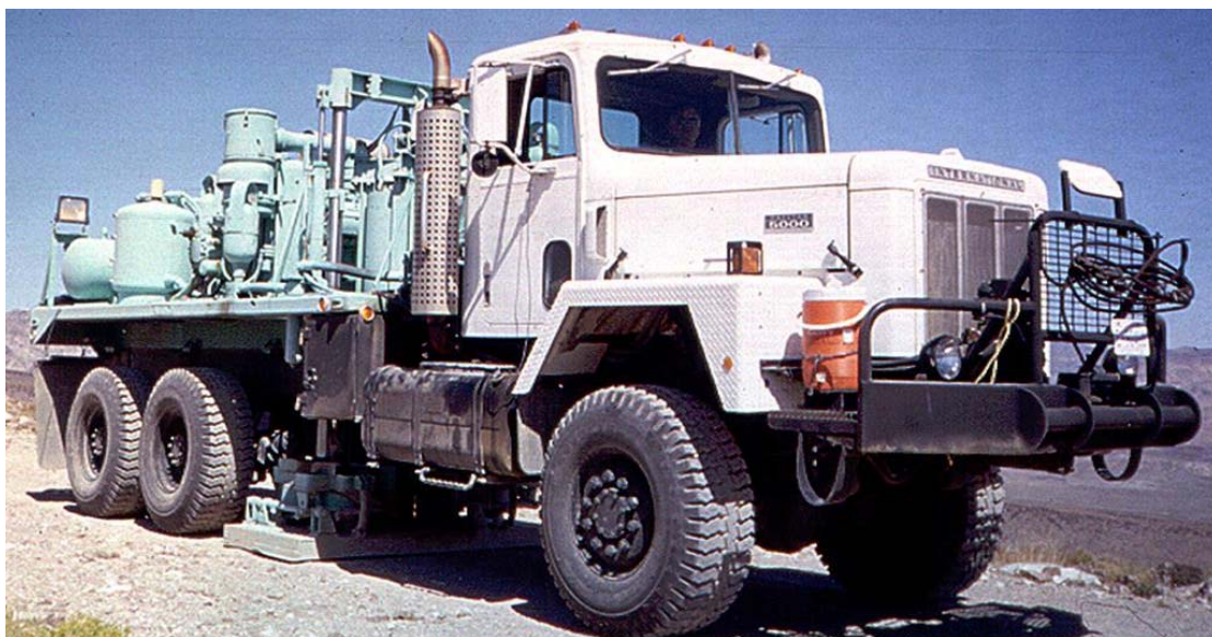
Figure 3 Photograph of Vibroseis truck in operation on the top of Yucca Mountain
