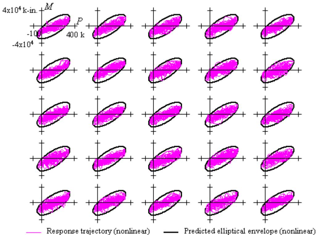
**Figure 8. Response trajectories, axial load-bending moment, location A.**
