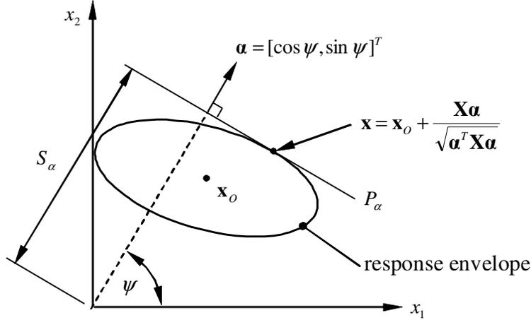
**Figure 1. Specification of the coordinates of a response-spectrum-based envelope.**
