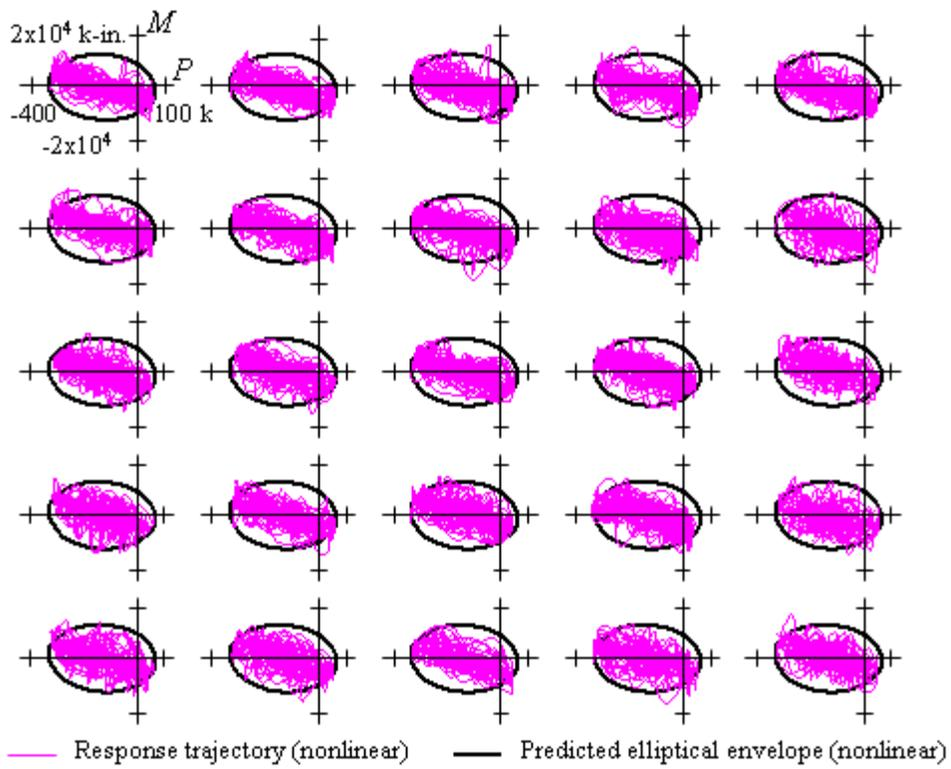
**Figure 9. Response trajectories, axial load-bending moment, location B.**
