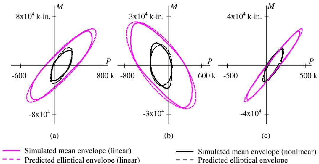
**Figure 7. Axial load-bending moment comparisons, simulated vs. predicted, locations A, B & C.**
