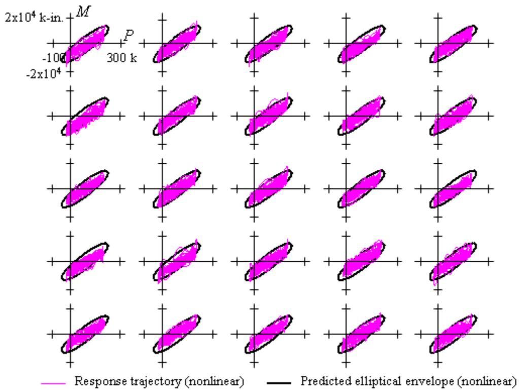
**Figure 10. Response trajectories, axial load-bending moment, location C.**
