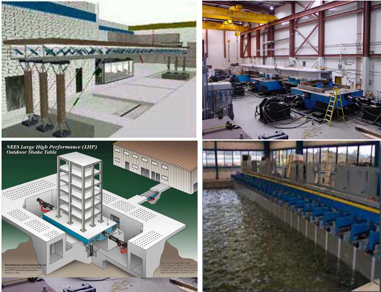
Figure 2. NEES Experimental Facilities (from upper left, clockwise): SUNY Buffalo - Dual Relocatable 6DOF Shake Tables; University of Nevada, Reno – Three Relocatable Biaxial Shake Tables; Oregon State University - Tsunami Wave Basin; and University of California, San Diego – Large High Performance Outdoor Shake Table.
