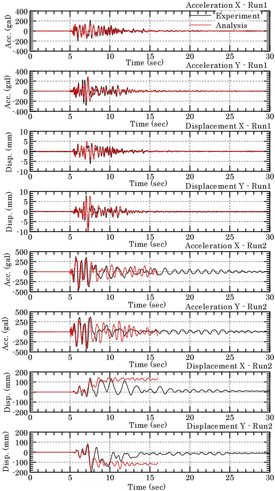
Figure-3 (1) Time histories of RA and RD at the center of inertia (Square cross section)
