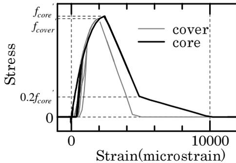
Figure-7 stress-strain relationship (concrete)
