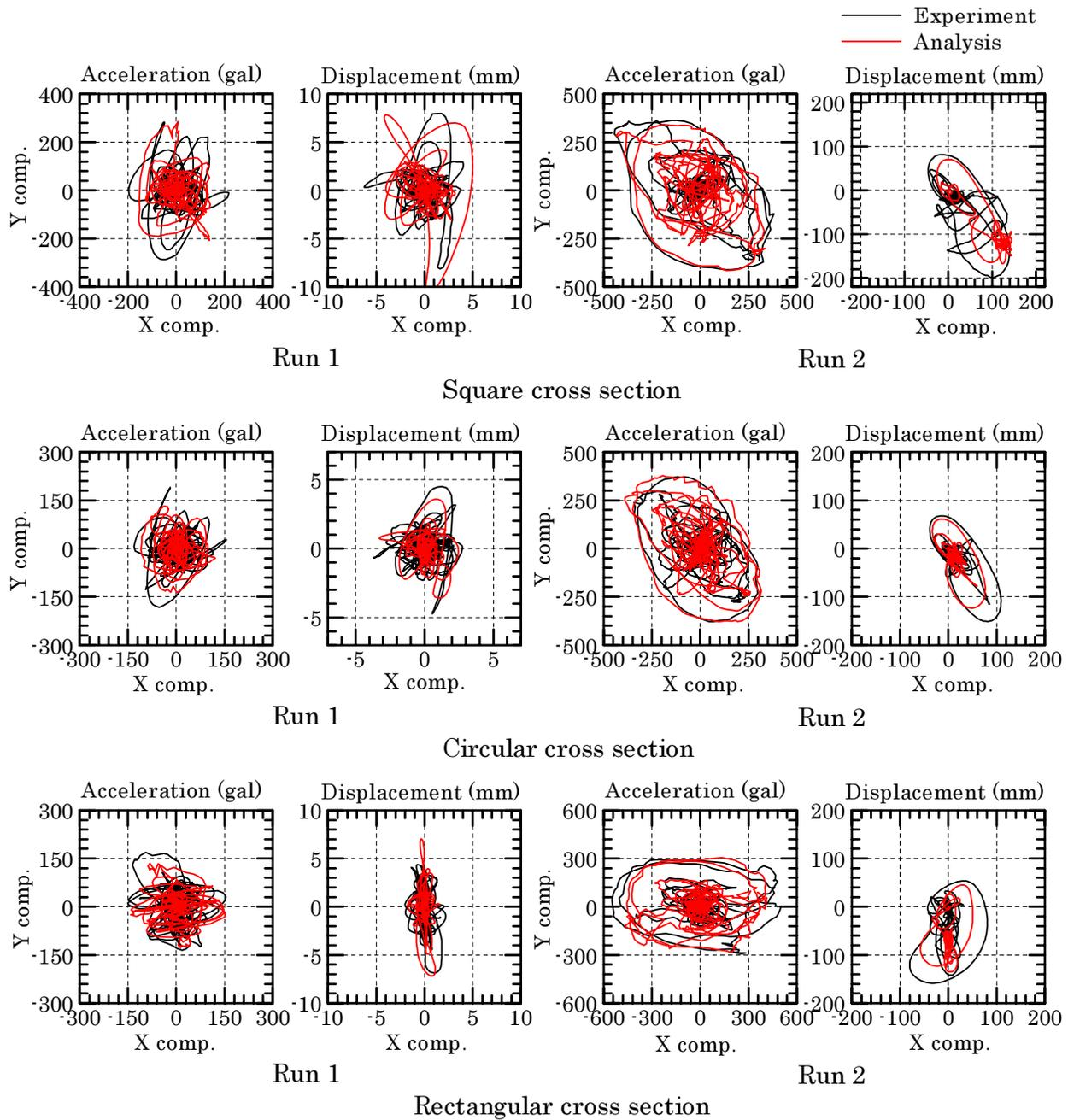
**Figure-4** Orbits of RA and RD at the center of inertia
