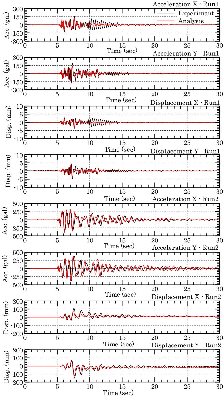
**Figure-3 (2) Time histories of RA and RD at the center of inertia (Circular cross section)**
