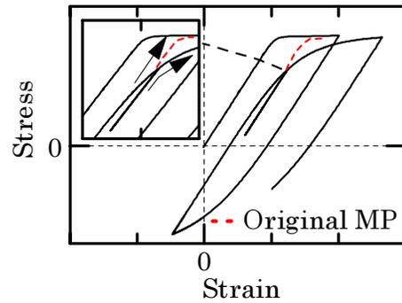
Figure-8 stress-strain relationship (steel bar)
