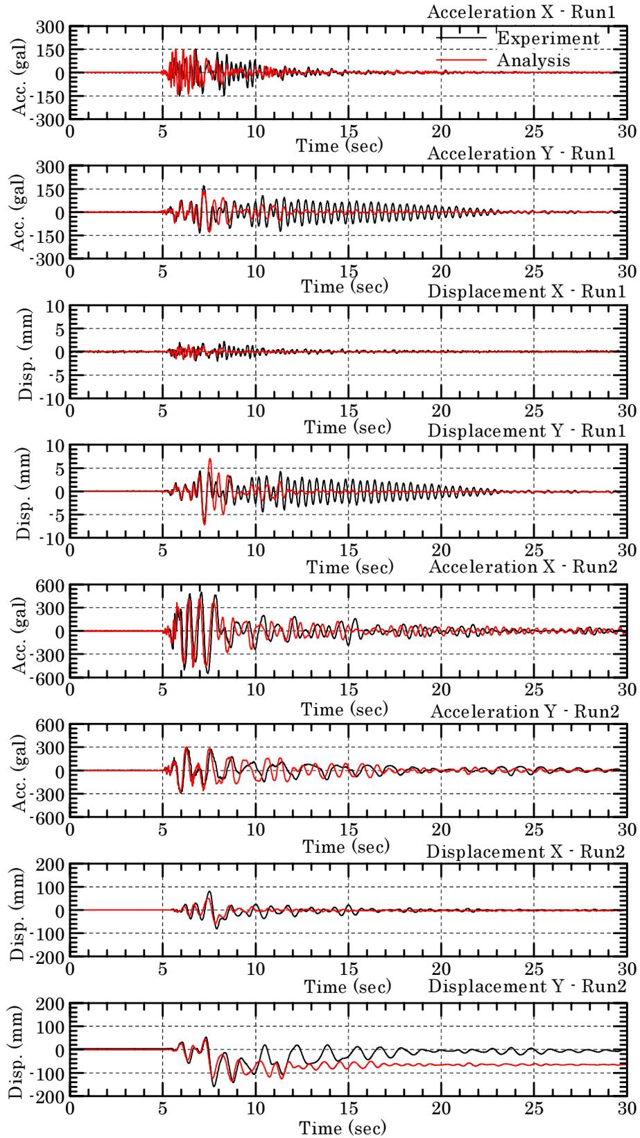
Figure-3 (3) Time histories of RA and RD at the center of inertia (Rectangular cross section)
