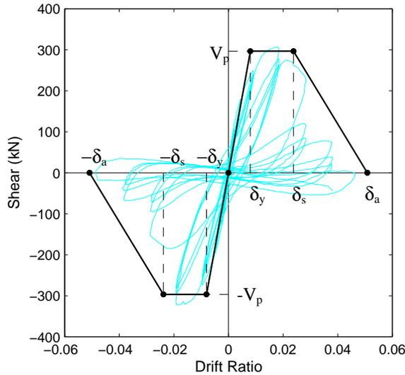
**Figure 2. Calculated idealized backbone plotted with column test data (Column data from reference [4])**
