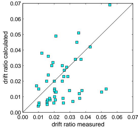
**Figure 4. Measured versus calculated drift at shear failure, interpreted from Sezen shear strength model.**
