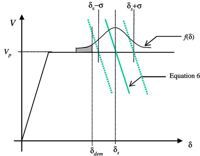
**Figure 16. Illustration of the application of a probabilistic capacity model for the drift at shear failure**
