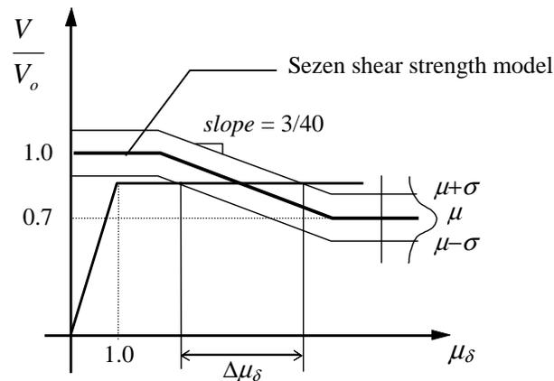
**Figure 3. Displacement at shear failure as function of model variability**
