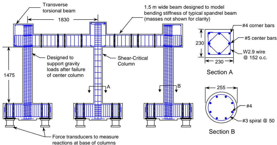
Figure 9. Shake table test specimen (units in mm).
