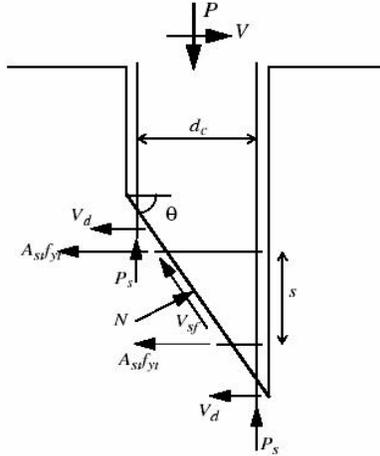
**Figure 6. Free-body diagram of column after shear failure**
