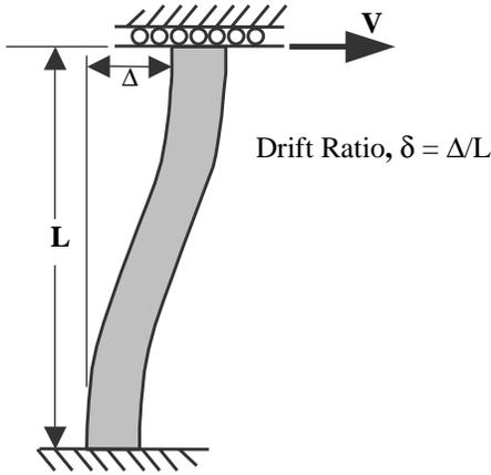
**Figure 1. Fixed-fixed column subjected to lateral loads**
