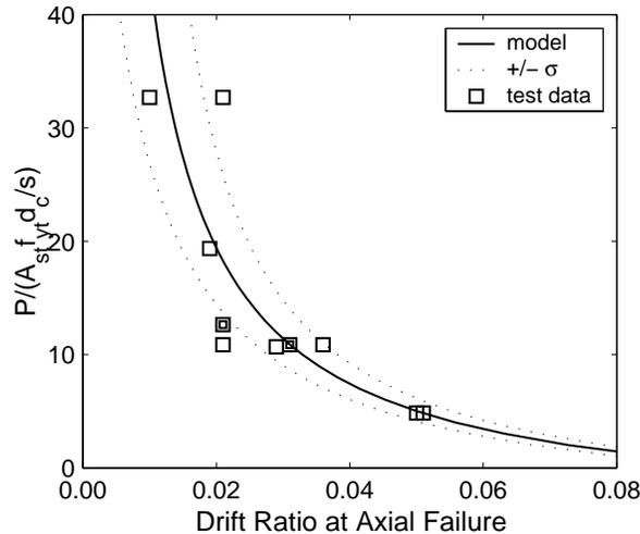
**Figure 7. Drift capacity curve based on shear-friction model**
