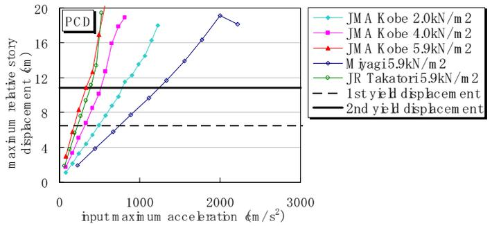
Fig. 8 Load-displacement relations
