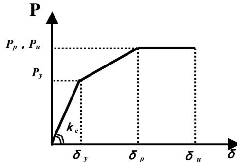
Fig. 7 Restoring force characteristics
