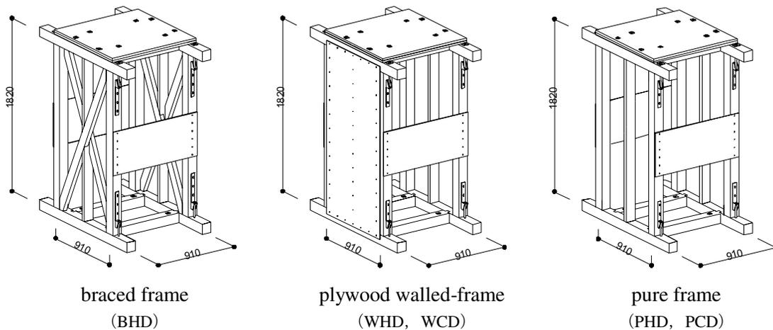
Figure 1 Test specimen (unit: mm)
