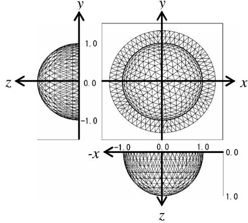
**Fig.1 Boundary element model for the irregular surface  $S_I$ .**
