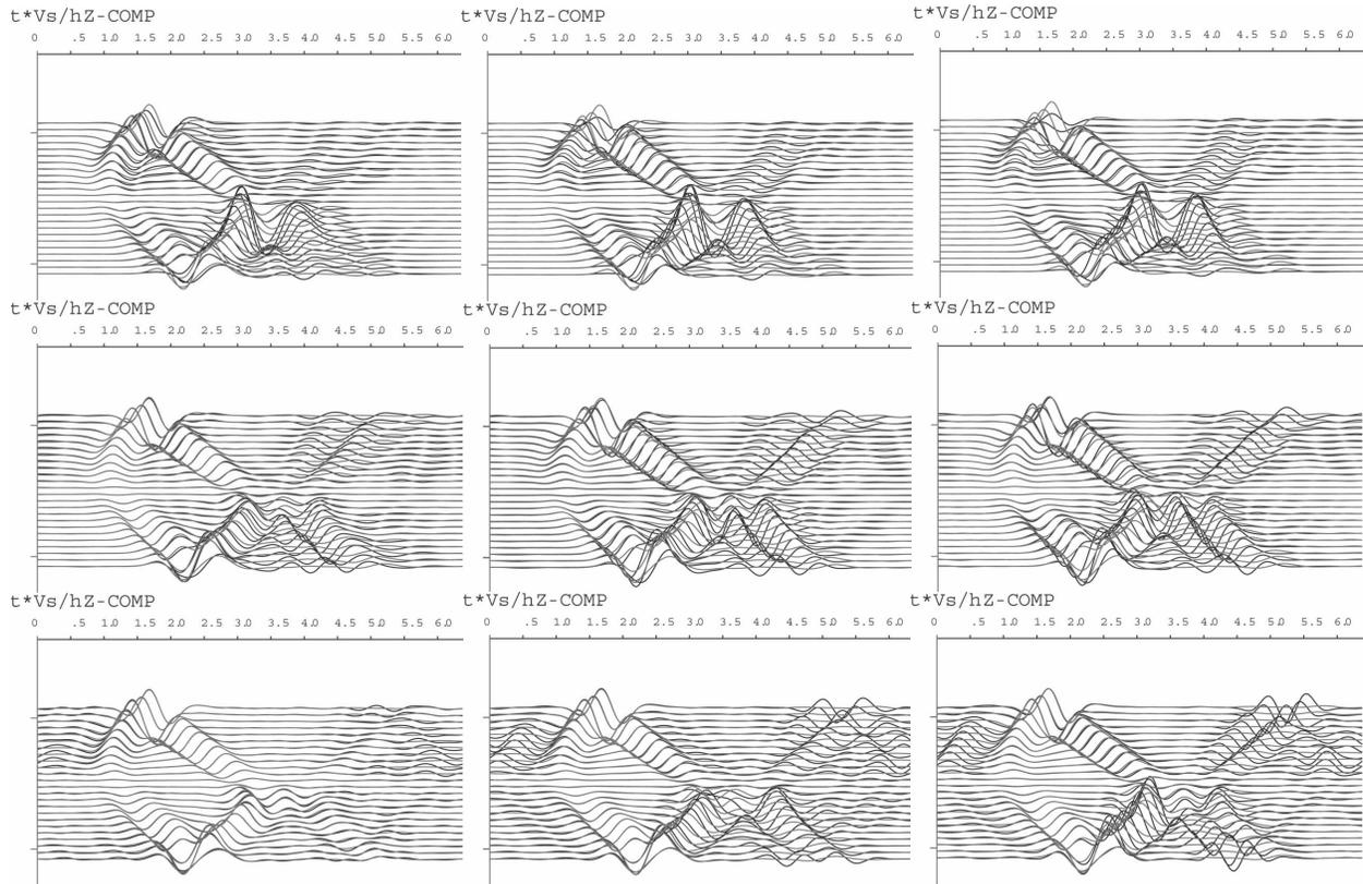
**Fig. 2** Solution with elimination of small elements (*left:  $\varepsilon = 0.1$ , center:  $\varepsilon=0.2$ , right:  $\varepsilon=0.5$* ). *Top: zero order, middle: first order, bottom: third order* Born approximation applied. Vertical components observed along the line  $x=y$  are shown. Ticks on the vertical axis show the edge of the semi-spherical canyon. Grey traces denote “the exact solution”, *i. e.*, the full matrix solution ( $\varepsilon=0.0$ ).
