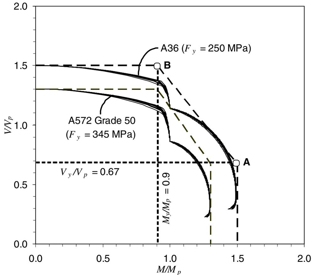
Figure 3: Normalized  $V$ - $M$  interaction surfaces for AISC  $W$ -sections with idealized upper bound for minimum specified yield strength and  $F_u/F_y = 1.5$  ( $F_y = 250$  MPa) and  $F_u/F_y = 1.3$  ( $F_y = 345$  MPa), and  $R_y = 1.0$ .
