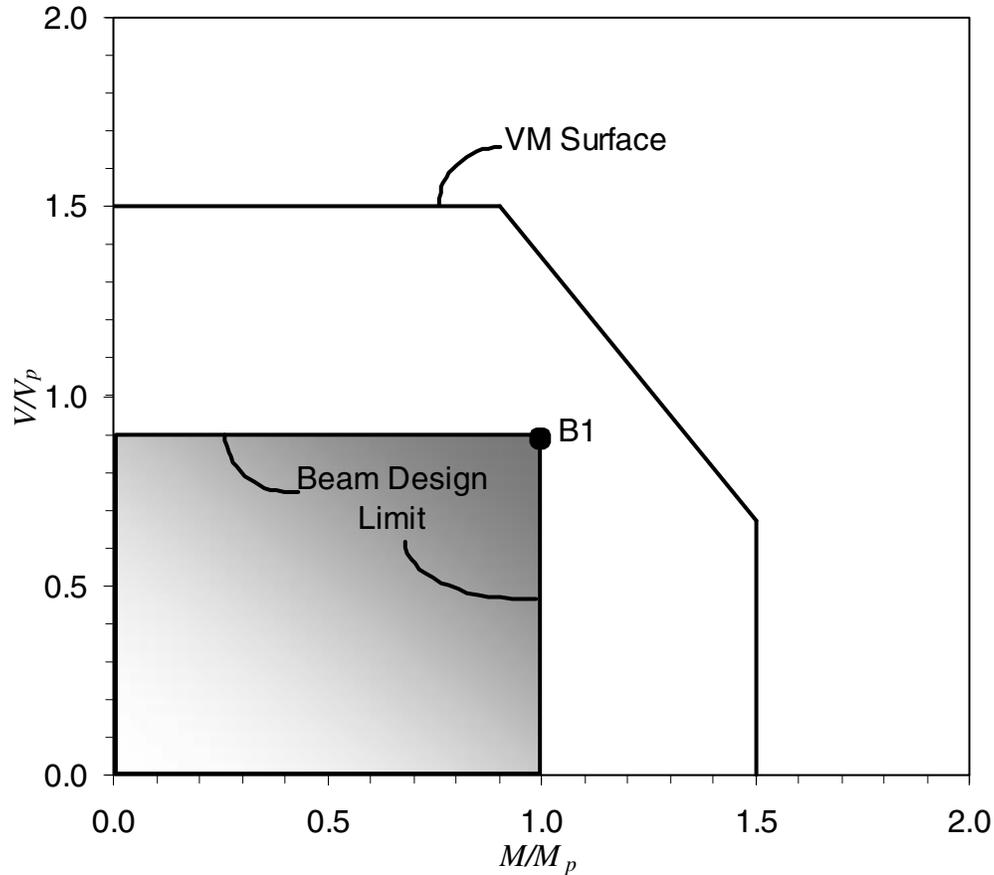
Figure 5: Idealized limiting  $V$ - $M$  interaction curve for design of beam-to-column connections with minimum specified yield strength and  $F_u/F_y = 1.5$  (for A36 steel) compared with the design limits employed in the existing beam design procedures.
