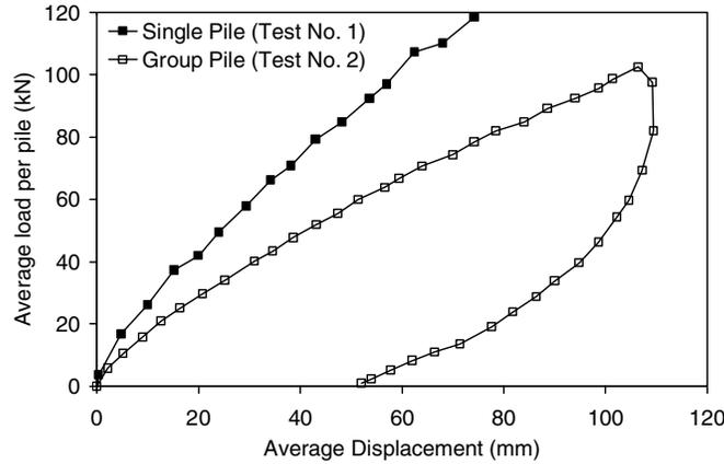
Figure 3 Measured load-displacement curves of single and group piles during static tests
