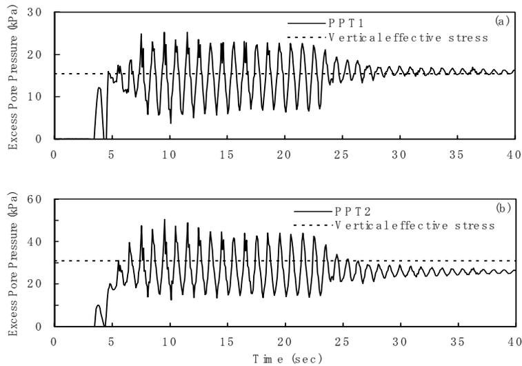
Figure 9 Measured excess pore water pressures at group pile test (Test No.6); (a) GL-2m, (b) GL-4m
