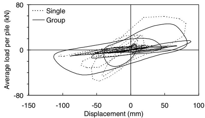
Figure 10 Measured load–displacement curve of group pile at dynamic test in saturated deposit (Test Nos.4 & 6)
