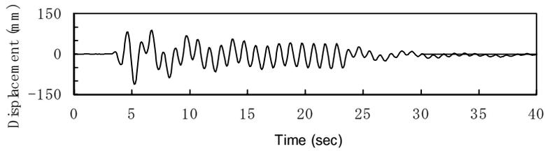
Figure 8 Measured displacement of pile head at dynamic test of group pile in saturated deposit (Test No.6)
