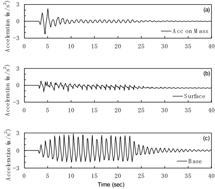
Figure 7 Measured accelerations of dynamic test of group pile in saturated sand deposit (Test No.6); (a) at pile head, (b) at model ground surface, and (c) input.
