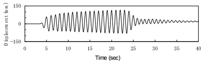
Figure 5 Measured displacement of pile head at dynamic test of group pile in dry deposit (Test No.5)
