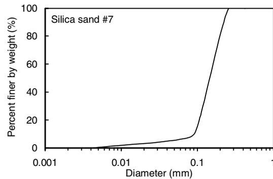
Figure 1 Particle size distribution of Silica sand #7
