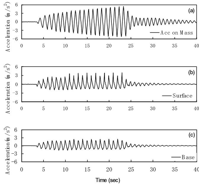
Figure 4 Measured accelerations of dynamic test of group pile in dry deposit (Test No.5); (a) at pile head, (b) at model ground surface, and (c) input.
