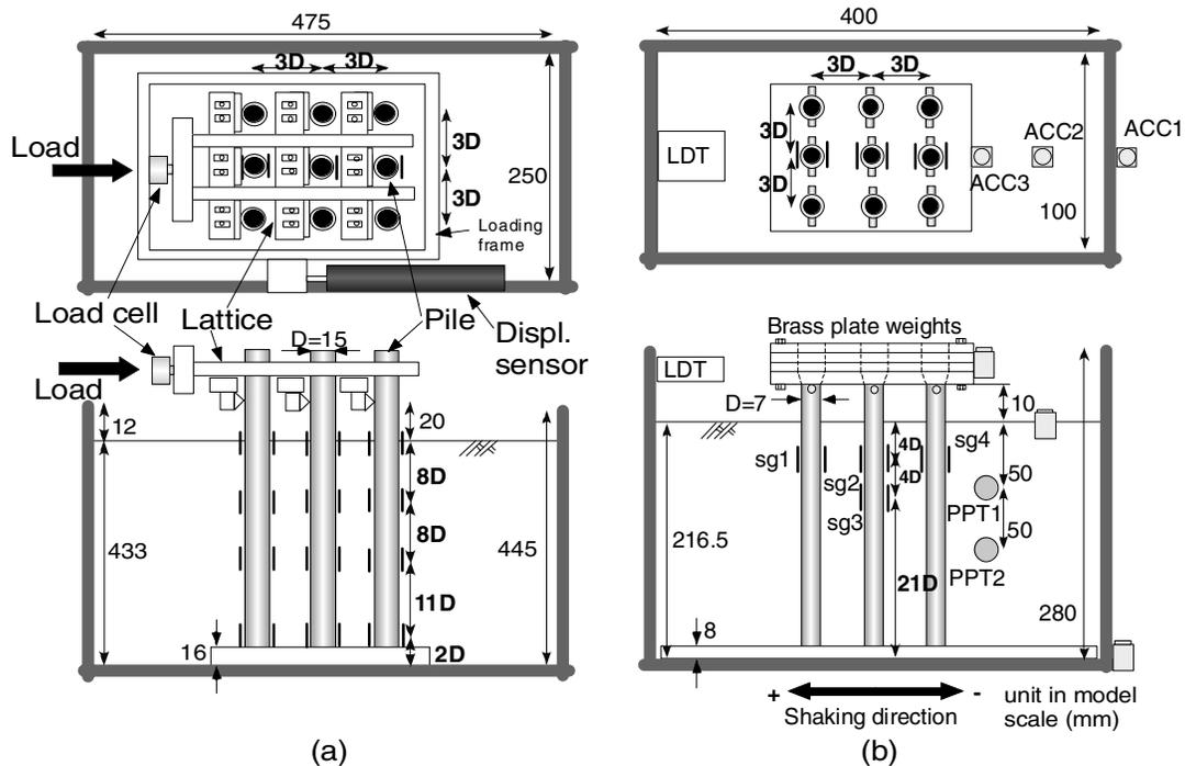
Figure 2 Cross section of model for (a) static test (Test No.2) and (b) dynamic test (Test No.6), Unit is in model scale
