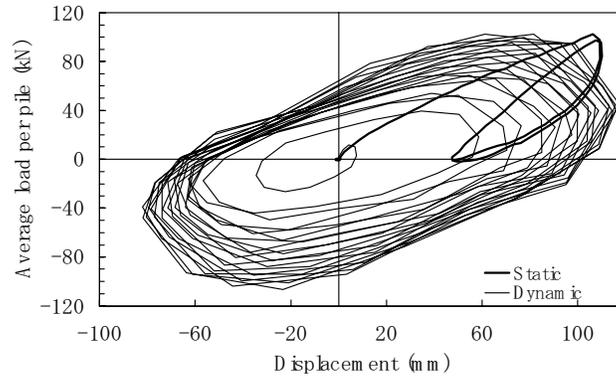
Figure 6 Static and dynamic load–displacement curves of group pile (Test Nos.2 & 5)
