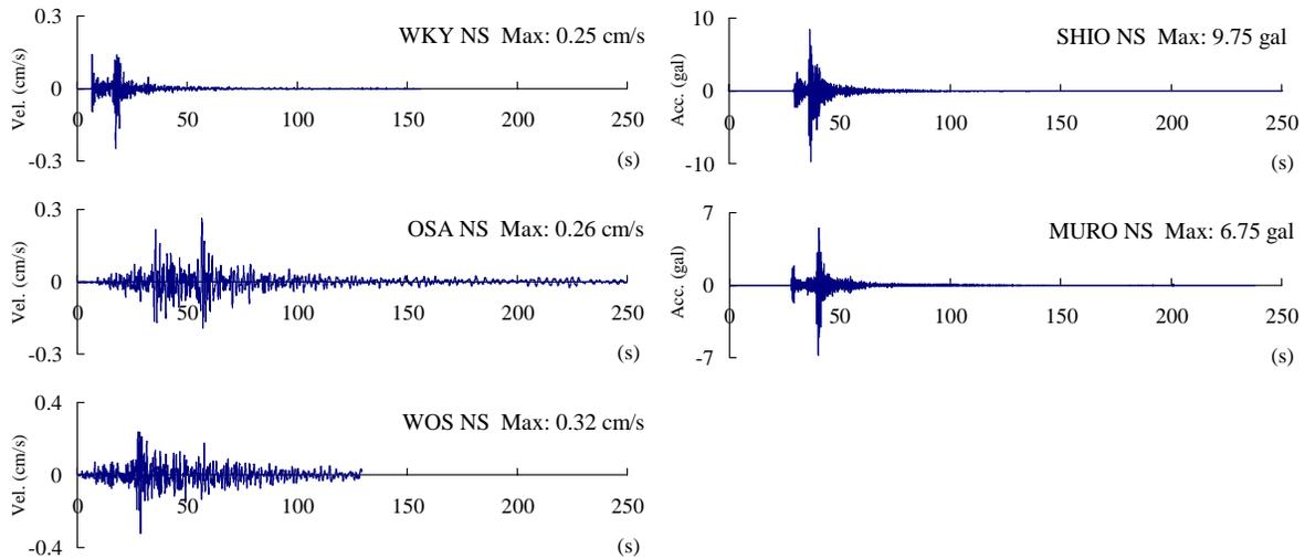
Fig. 2 Acceleration and velocity waveforms used as the empirical Green's functions
