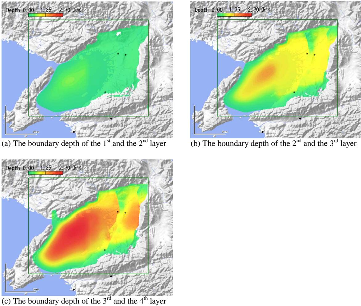
Fig. 9 Depth distribution of each sediment layer in 3-dimensional model of the Osaka basin.
