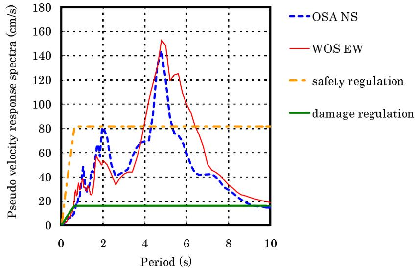
Fig. 4 Pseudo velocity response spectra of the predicted ground motions for the Nankai earthquake at OSA and WOS sites located inside the Osaka basin. A couple of the design spectra are depicted in this figure.
