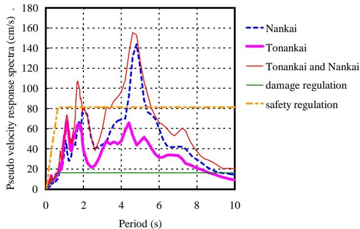
Fig. 8 Pseudo velocity response spectra of the predicted ground motions at OSA site in cases of the individual occurrence of the Nankai and the Tonankai earthquakes and the linked occurrence of both earthquakes. A couple of the design spectra are depicted in this figure.
