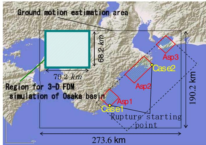
Fig. 10 Map showing the region for calculating long period ground motions from the Tonankai earthquake. The thick rectangular box depicts the region for the 3-D simulations. The dotted line and the red lines indicate fault area and asperities, respectively.
