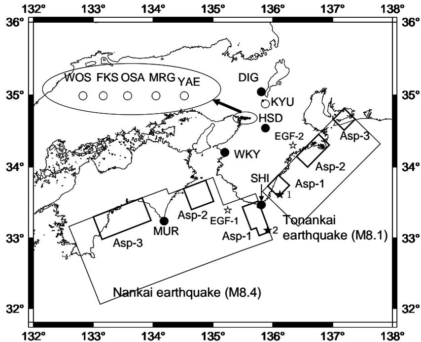
Fig. 1 Map showing the source model composed of three asperities on the fault for the Nankai and the Tonankai earthquakes and site locations. EGF-1 and EGF-2 are the epicenters of earthquakes used as the empirical Green's functions for the Nankai and the Tonankai earthquakes, respectively.
