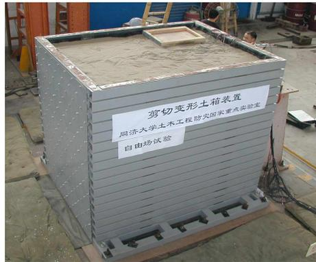
Fig.9 Shear deformation soil box
