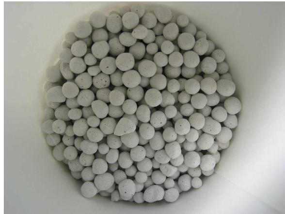
Photo. 2 Lightweight glass aggregate (Type : L)
