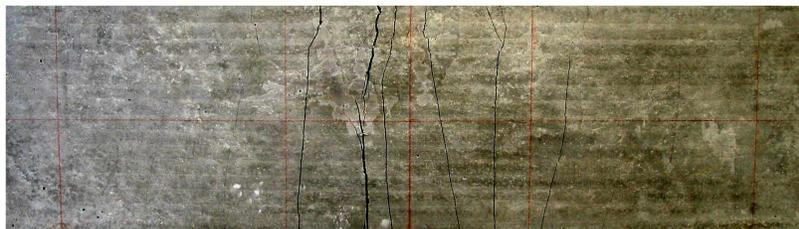
Photo. 3 An example of a typical cracking pattern on the bottom for the specimen
