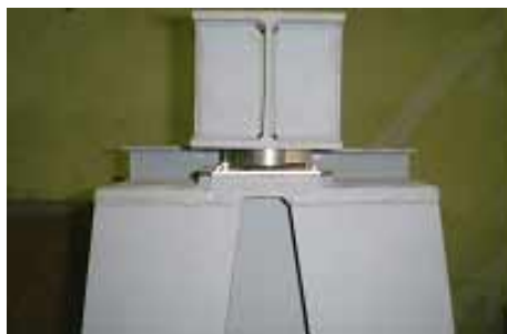
Fig.8 Spherical Bearing (unit : mm)
